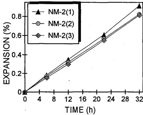
Figure 4 Expansion of rock prisms autoclaved at 150°C in 10% KOH solution.
