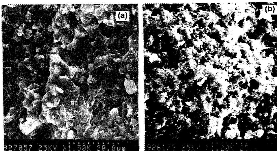
Figure 8 The central part of the MN-2 prism (a) before and (b) after autoclaving at 150°C in 10 % KOH solution
