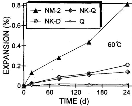
Figure 5 Expansion of concrete microbars cured at 60°C in 10% KOH solution
