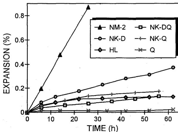
Figure 2 Concrete microbar expansion of the selected rocks
