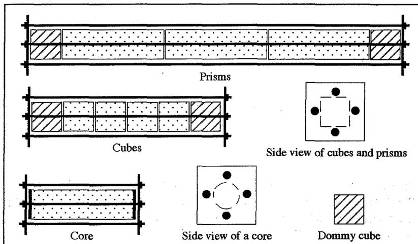
*Fig. 1 - Method of applying external restraint on various specimens.*
