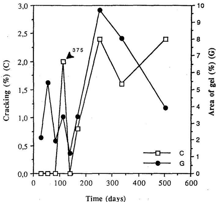
Fig. 5 Graph of cracking vs. area occupied by gel (%).
