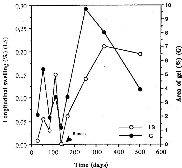
Fig. 4 Graph of longitudinal swelling vs. surface area occupied by gel (%).
