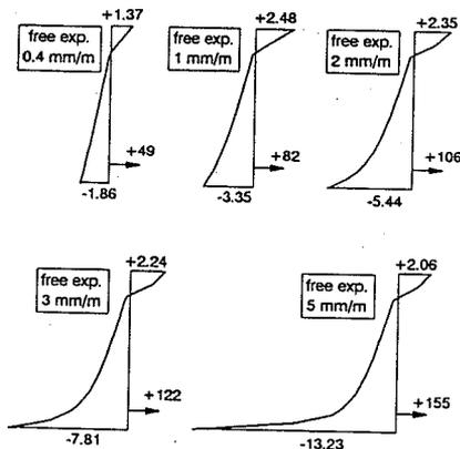
Fig. 5. Predicted stress distributions across the sections of the singly reinforced beam tested by Cope et al, without loading during conditioning. Arrow represents reinforcement stress. Stress unit  $N/mm^2$ . Sign: + tension; - compression.
