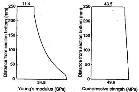
Fig. 6 Estimated Young's modulus and compressive strength through the section of singly reinforced beam conditioned unloaded.
