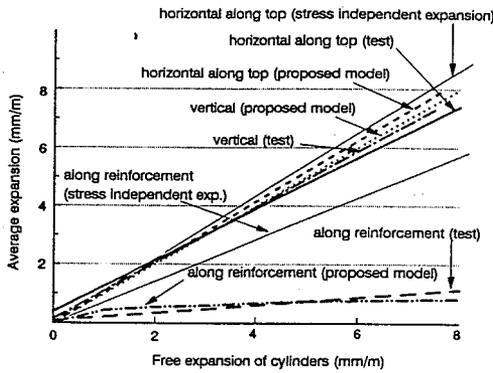
Fig. 4 Comparison of expansion measurements with the predicted values using the proposed model and with those using elastic analysis assuming the expansion stress independent.
