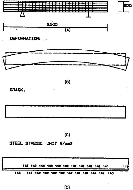
Fig. 3 A) Finite element model for the singly reinforced beam.
