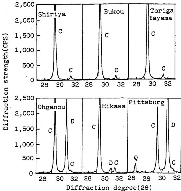
Fig.5 The diagram of X-ray diffraction of limestone aggregate samples (C:Calcite, D:Dolomite, Q:Quartz)
