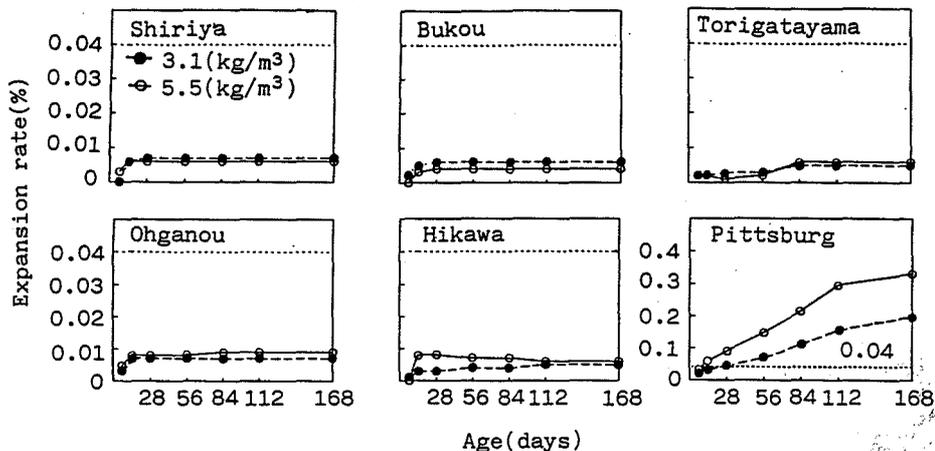
Fig.6 Variation of expansion rate versus time
