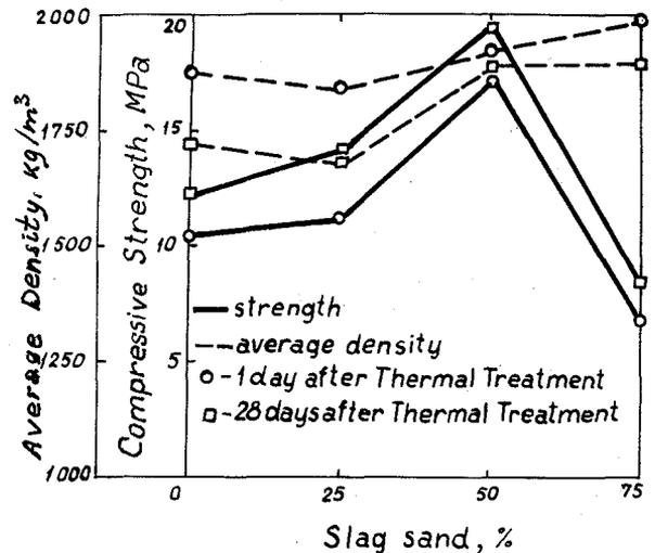
Fig.4. Compressive strength of cementless ash concrete versus the amount of slag sand
