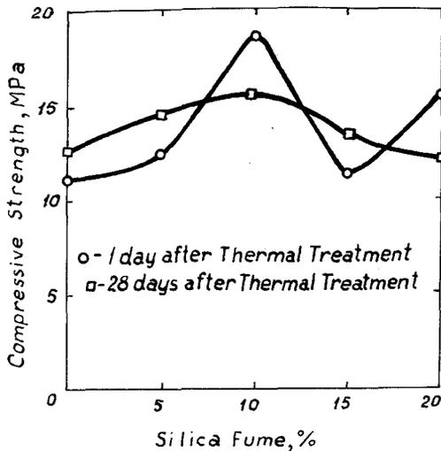
Fig.3. Compressive strength of cementless ash concrete versus the amount of silica fume
