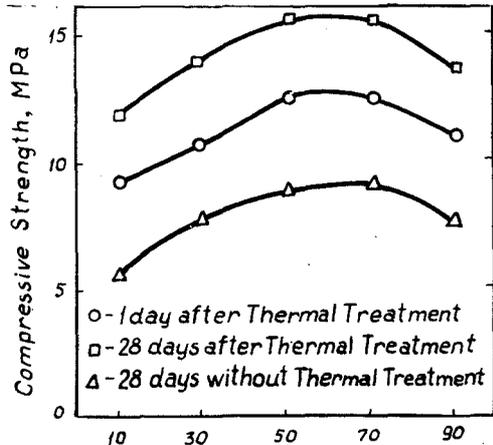
Fig.2 Compressive strength of cementless ash concrete versus the temperature of mixing water (°C)
