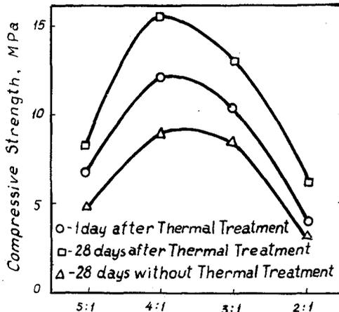
Fig.1 Compressive strength of cementless concrete versus ash-to-water ratio (A/W)
