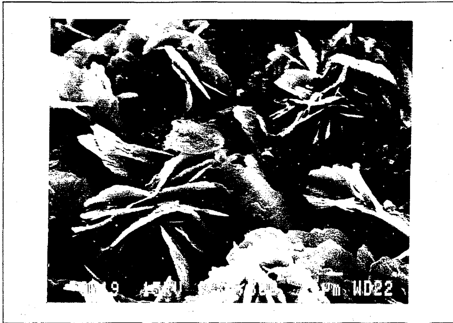
Fig. 4 SEM micrograph - Detail at high magnification. Strips of minerals developed on the surface of the gel
