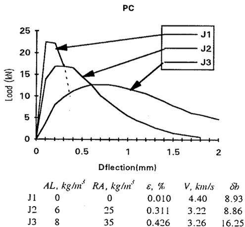
Fig. 5 Influence of AAR on Load-Deflection Curve of Plain Concrete
