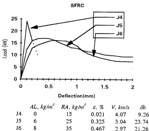
Fig.6 Influence of AAR on Load-Deflection Curve of SFRC ( $V_f=0.5\%$ )
