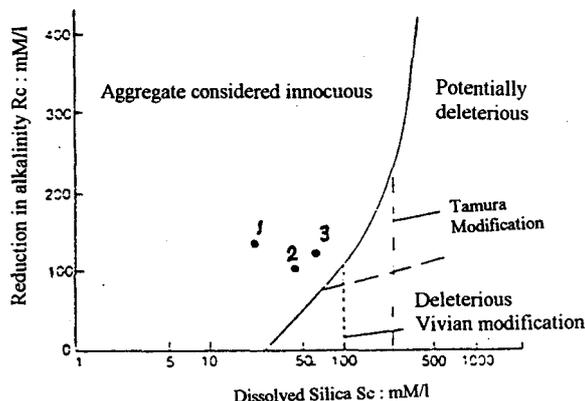
Fig1 : Results of ASTM C 289 chemical test for the Rajai dam aggregates.
