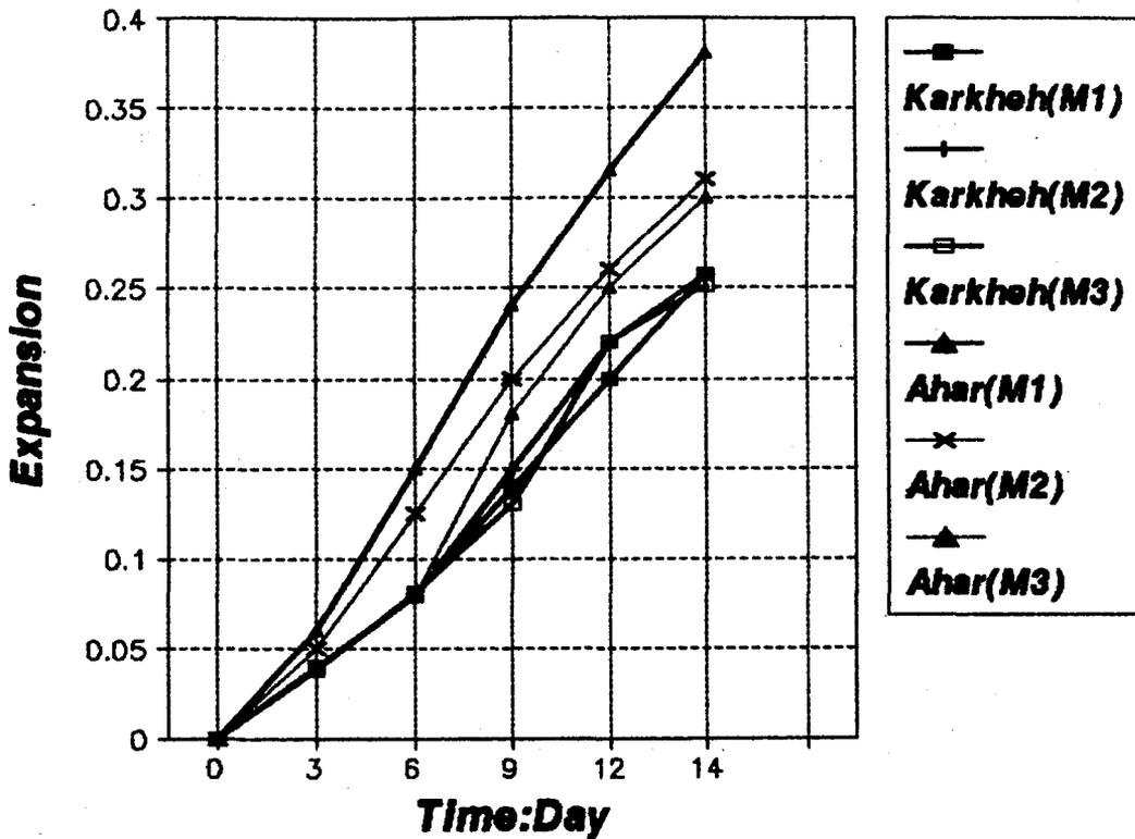
Fig5 :Results of the CSA accelerated Mortar bar testing of 3. Karkheh ; 4. Ahar aggregates According to CSA A23.2-25A.
