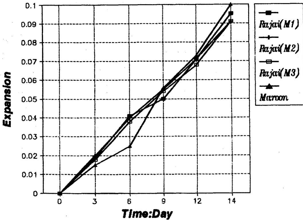
Fig4 : Results of the CSA accelerated Mortar bar testing of 1) shaid rajaii ; 2) Maroon aggregates According to CSA A23.2-25A.
