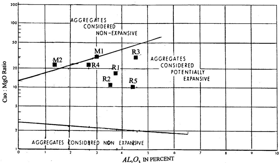
**Fig2 : Results of the CSA A 23.2-26A chemical test**
