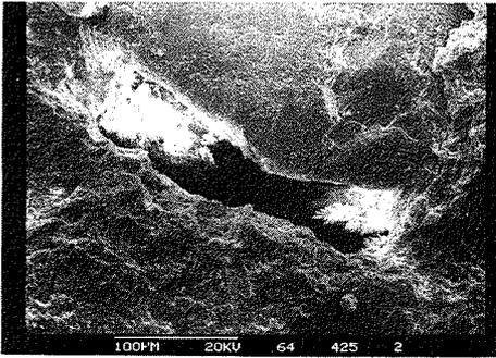
**Fig. 4.** Scanning electron micrographs showing various morphological features of ettringite at cement/aggregate interfacial zones. The lower left micrograph shows a gap at the interface partially filled with ettringite.
