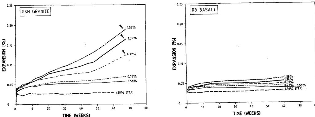
Fig. 9. Expansion curves for concrete blocks stored in water at 50°C. Numbers on the curves indicate cement alkali level. Cement content of concrete was 410 kg/m<sup>3</sup>. TFA indicates 25% fly ash replacing cement on mass basis. Arrows indicate when cracking was noted.
