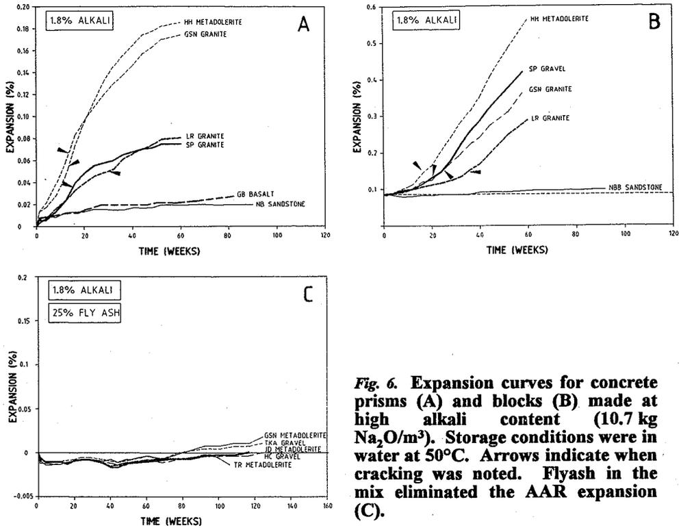
**Fig. 6. Expansion curves for concrete prisms (A) and blocks (B) made at high alkali content (10.7 kg Na<sub>2</sub>O/m<sup>3</sup>). Storage conditions were in water at 50°C. Arrows indicate when cracking was noted. Flyash in the mix eliminated the AAR expansion (C).**
