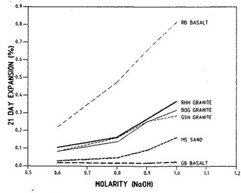
**Fig. 7. Results of accelerated testing of mortar bars made with the various aggregates at different Na OH concentrations (80°C).**
