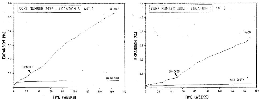
**Fig. 5.** Expansion curves for cores under the two different storage conditions. Cores from locations 1, 2, 4 and 5 behaved similarly to those from location 3 (left). Cores from location 7 expanded half those from location 6 (right).
