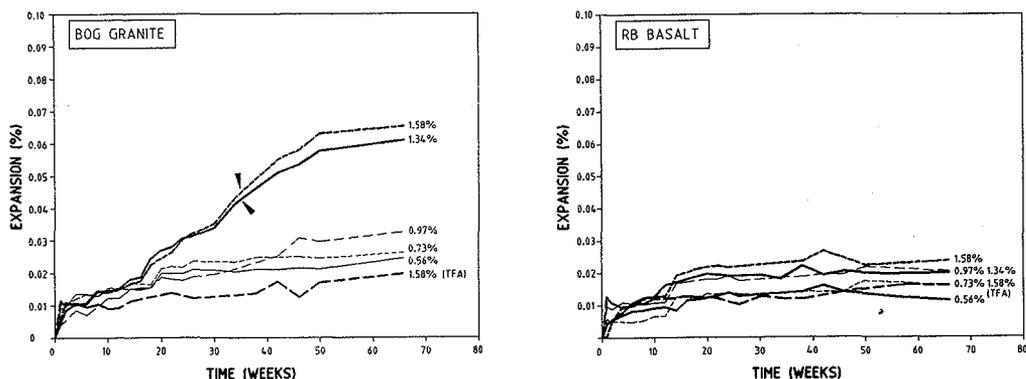
Fig. 8. Expansion curves for concrete prisms made at different alkali contents and stored at 40°C, 100% RH. Arrows indicate when cracking was noted.
