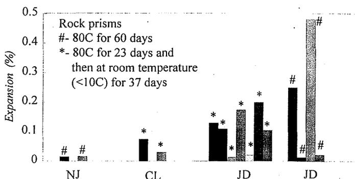
Fig. 1 Expansions of rock prisms cut from the coarse aggregates
