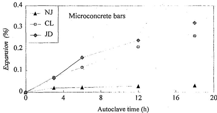
Fig. 2 Expansion of microconcrete bars vs. autoclave time
