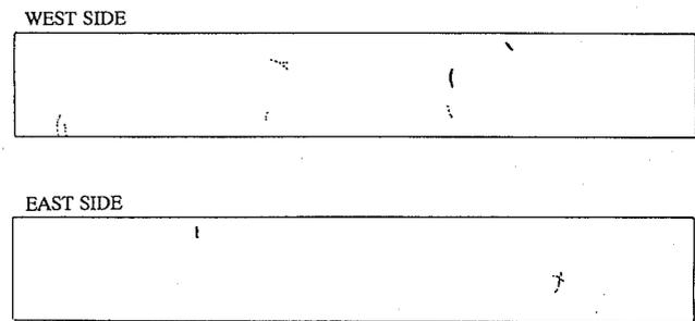
Fig. 6 Cracking patterns of PC mixture without the additional alkali ( 2.6 kg/m<sup>3</sup> Na<sub>2</sub>O eq., 50 mA/m<sup>2</sup> ).
