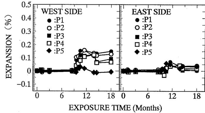
Fig. 9 Expansive behaviors of RC mixture with the additional alkali ( $4.7 \text{ kg/m}^3 \text{ Na}_2\text{O eq.}, 50 \text{ mA/m}^2$ ).
