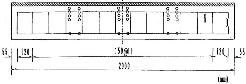
Fig. 1 Dimensions of the reinforced concrete beam used.
