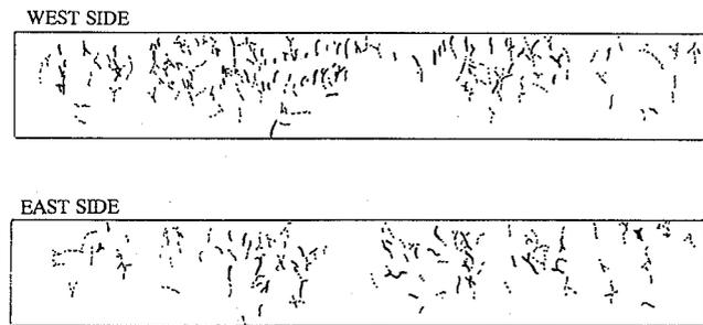
Fig. 7 Cracking patterns of PC mixture with the additional alkali ( 5.0 kg/m<sup>3</sup> Na<sub>2</sub>O eq., 50 mA/m<sup>2</sup> ).
