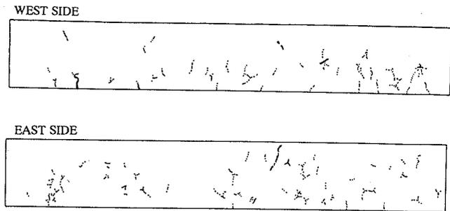
Fig. 4 Cracking patterns of RC mixture without the additional alkali ( 2.3 kg/m<sup>3</sup> Na<sub>2</sub>O eq., 50 mA/m<sup>2</sup> ).
