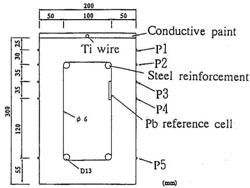
Fig. 2 Cross-section of the reinforced concrete beam used.
