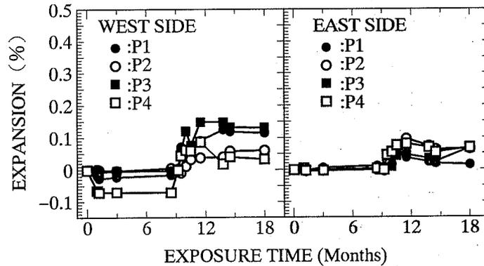
Fig. 10 Expansive behaviors of epoxy-resin coated RC mixture with the additional alkali ( $4.7 \text{ kg/m}^3 \text{ Na}_2\text{O eq.}, 50 \text{ mA/m}^2$ ).
