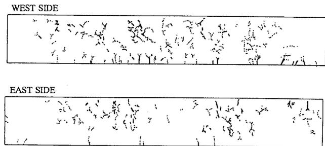
Fig. 5 Cracking patterns of RC mixture with the additional alkali ( 4.7 kg/m<sup>3</sup> Na<sub>2</sub>O eq., 50 mA/m<sup>2</sup> ).
