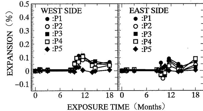
Fig. 11 Expansive behaviors of PC mixture with the additional alkali ( $5.0 \text{ kg/m}^3 \text{ Na}_2\text{O eq.}, 50 \text{ mA/m}^2$ ).
