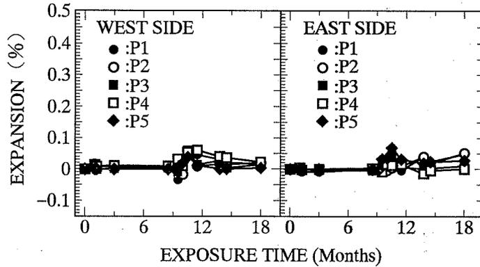
Fig. 8 Expansive behaviors of RC mixture without the additional alkali ( $2.3 \text{ kg/m}^3 \text{ Na}_2\text{O eq.}, 50 \text{ mA/m}^2$ ).
