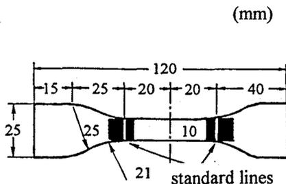
Fig. 3 Specimen for Elongation test.
