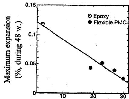
Fig. 10 Relation between water vapor permeability and ASR expansion (48 weeks)
