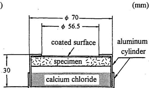
Fig. 2 Specimen for water vapor permeability test
