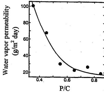
Fig. 6 Relation between P/C and water vapor permeability
