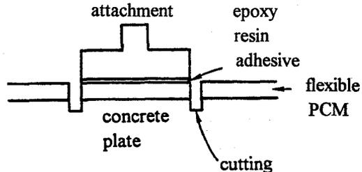
Fig. 4 Adhesive strength test
