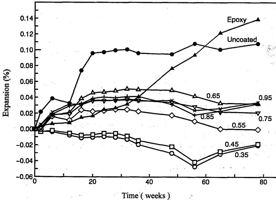
Fig. 9 Length change in field exposure test I
