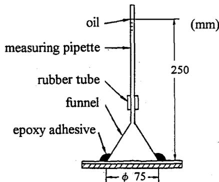
Fig. 1 Specimen for water permeability test
