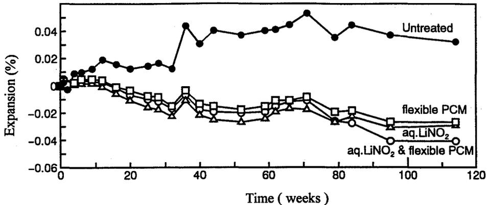
Fig. 11 Length change in field exposure test II
