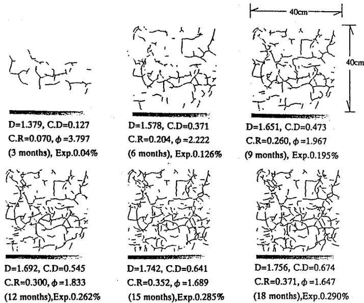
Fig. 11 Crack patterns at the several ages
