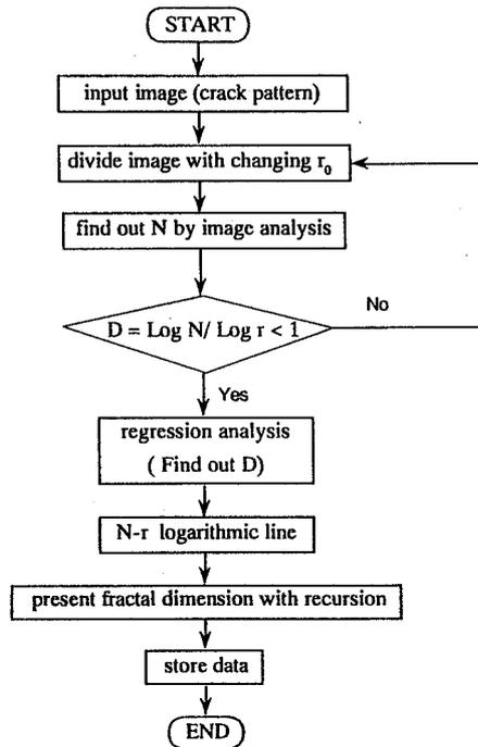
Fig. 2 System Flow of Fractal Dimension Analysis
