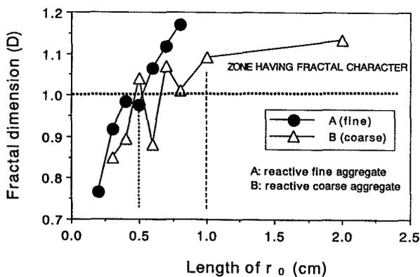
Fig. 7 Lower limit of  $r_0$
