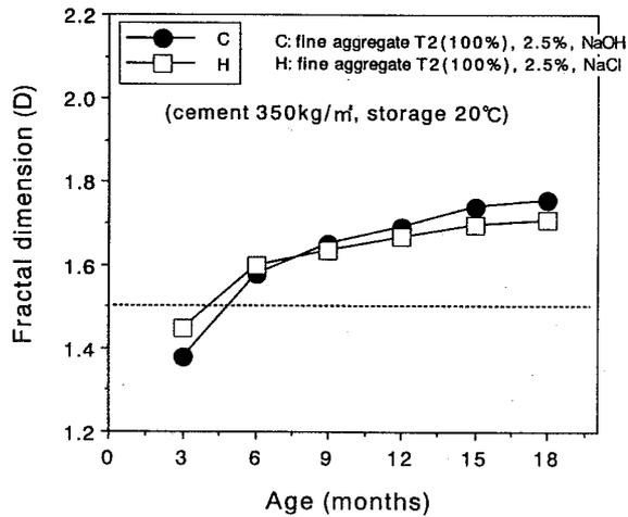
Fig. 10 Fractal dimension VS. time in 20°C, 100% RH. storage
