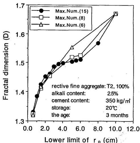
Fig. 6 Relationships between  $D$  and lower limit of  $r_0$ .
