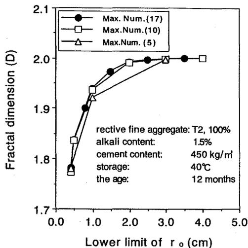
Fig. 5 Relationships between  $D$  and lower limit of  $r_0$ .
