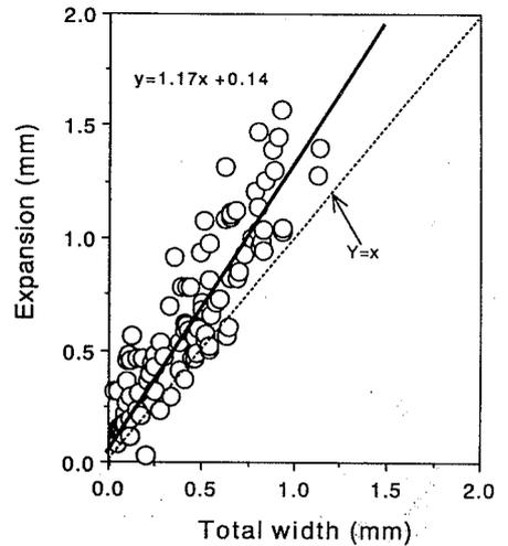
Fig. 9 Expansion and total width of cracks between the plugs
