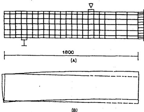
Fig. 2 (A) Finite element mesh. (B) Deformation at free expansion 5 mm/m.
