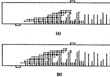
Fig. 5 Predicted crack pattern of (A) beam with AAR and (B) control beam.
