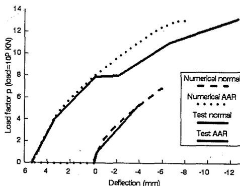
Fig. 3 Numerical and experimental load-deflection curves of the beam by Bach et al.
