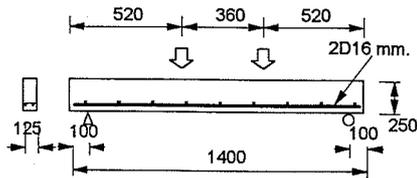
Fig. 6 Details of the beam for numerical studies.
