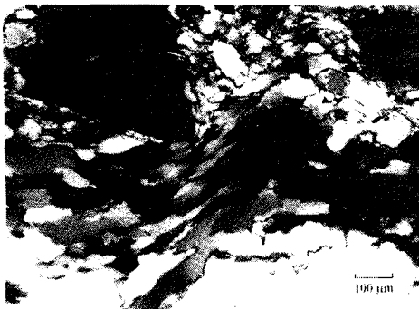
Fig. 1 Mylonite (Sample 1.3b). Intensive strain has produced these elongated quartz grains exhibiting undulatory extinction, sutured grain boundaries, and sub-grain development. Note the alignment in the area of most strain, around the porphyroclast (Polarised light).
