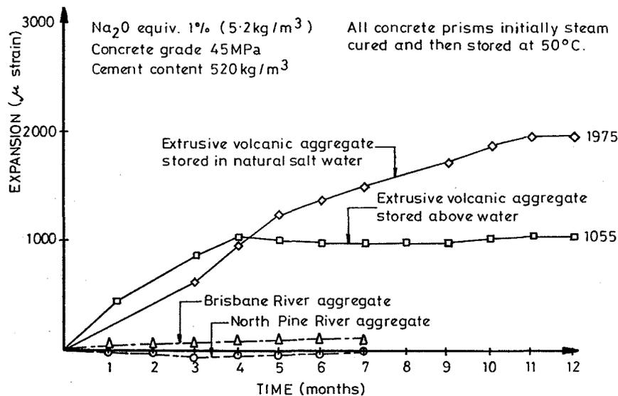
Fig. 7 Accelerated test on concrete for ASR
