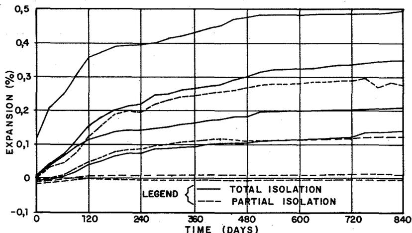
Fig.3- Concrete Expansion with Superficial Sealing
