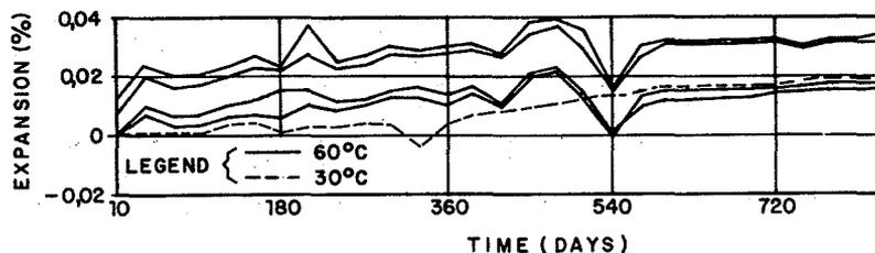
Fig.2- Concrete Expansion with Cores Taken from the Lower Part of the Structures
