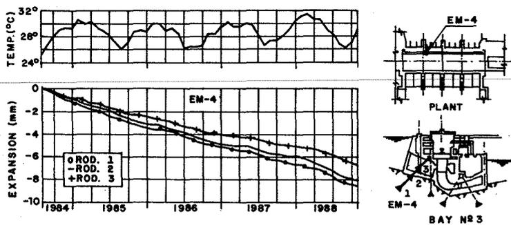
Fig.6- Concrete Expansion Measured by Extensometer EM-4
