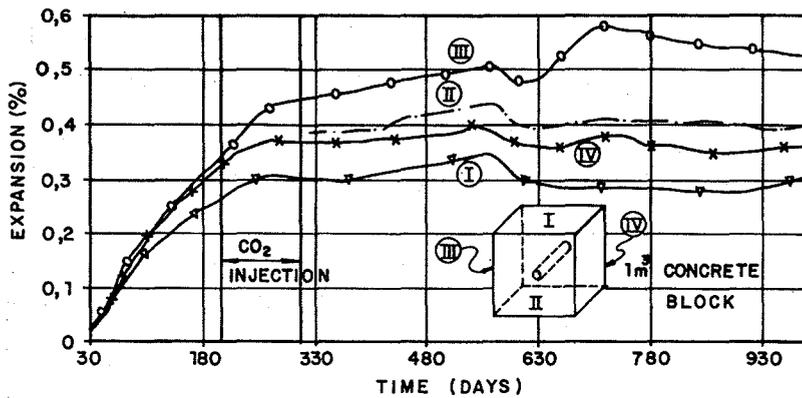
Fig.4- Effect of Carbonation on the Concrete Block Expansion
