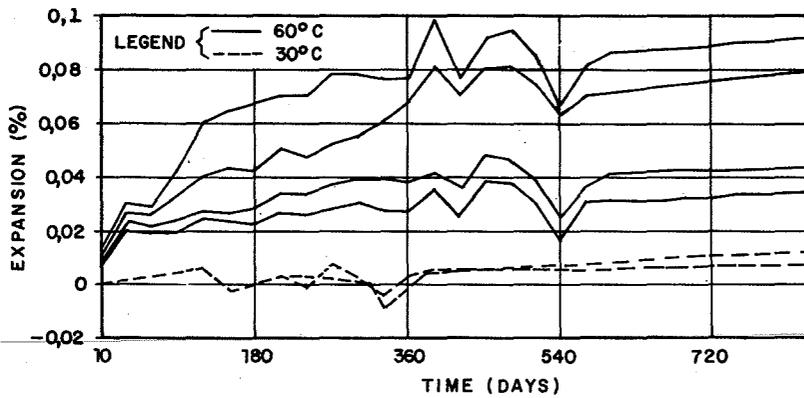
Fig.1- Concrete Expansion with Cores Taken from the Upper Part of the Structures
