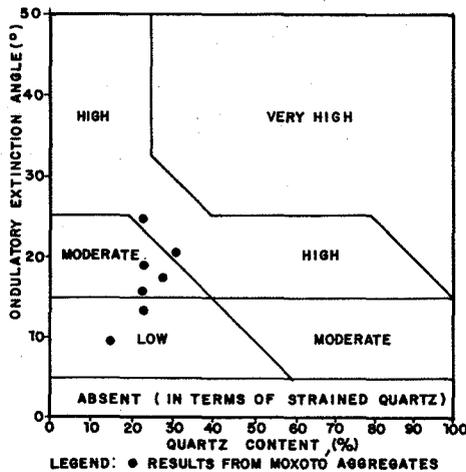
Fig.7- Reactivity of Aggregates with Strained Quartz Based on Usual Criteria
