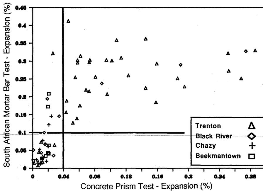
Figure 3. Expansion values at 14 days (Accelerated South African Mortar Bar Test) as a function of the expansions at 6 months (Concrete Prism Test)
