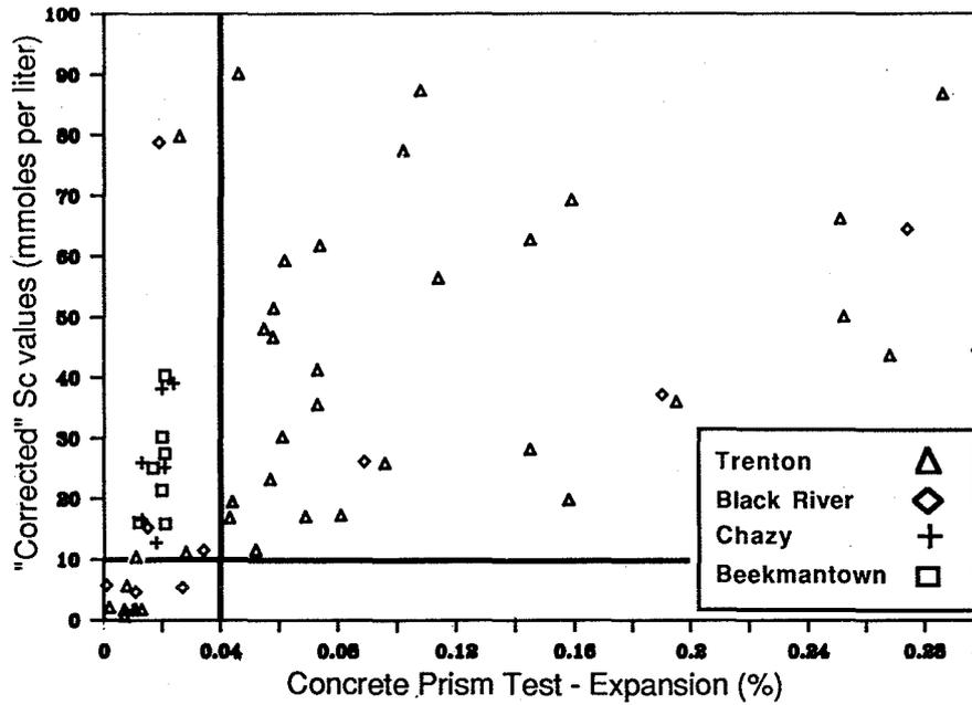
Figure 2. "Corrected" Sc values (mmoles per liter) as a function of the 6 month expansion values measured at the Concrete Prism Test.
