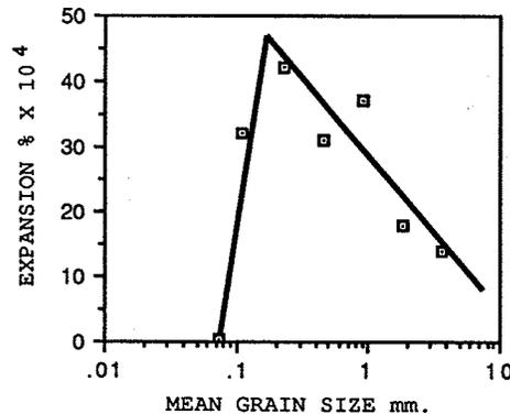
Figure 1. Effect of grain size of opal on expansion of mortar bars. After Kawamura [16].
