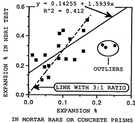
Figure 8. Comparison of expansions of mortar bars in the NBRI test, with results obtained using ASTM C227 or the concrete prism method by 3 laboratories. The outliers (circled) were excluded when the solid line was fitted to the points in the graph. The dashed line indicates the 3:1 ratio of expansion in the NBRI test : expansions in other methods.
