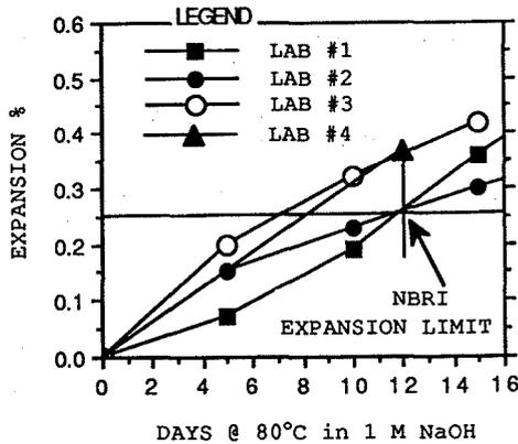
Figure 7 Expansions of mortar bars made with siliceous limestone aggregate in the NBRI test by four laboratories: #1 [51], #2 [52], #3 the author's and #4 [53]
