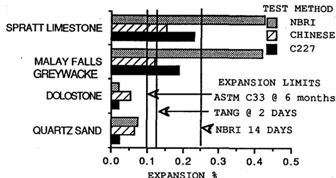
Figure 9. Comparison of expansions obtained with 2 reactive and 2 non-reactive aggregates using ASTM C227, the NBRI quick test and the Chinese autoclave method.
