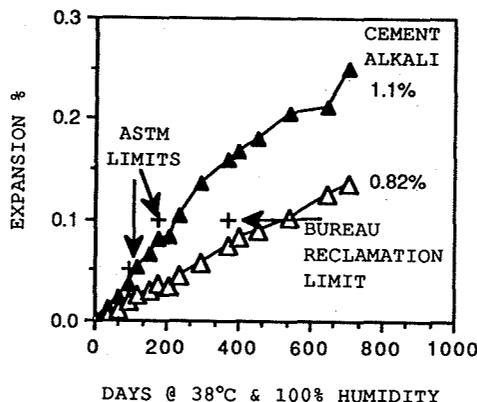
Figure 4. Effect of alkali content of cement on expansion of mortar bars made with slowly expanding Malmsbury aggregate. Data from Oberholster [31]
