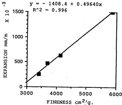
Figure 5. Effect of fineness of cement on expansion of concrete prisms. After Krell [28]
