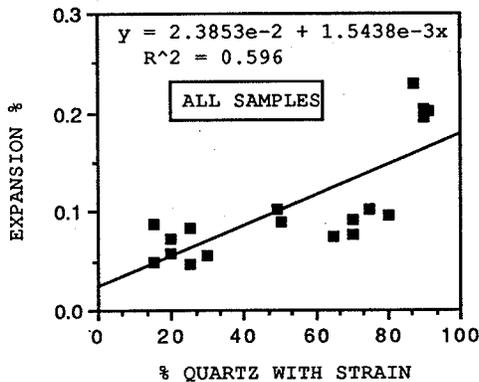
Figure 6a Influence of percentage of strained quartz in aggregate on the expansion of mortar bars. After Mullick [46]
