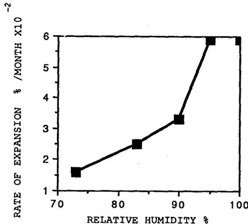
Figure 3. Effect of relative humidity on expansion of mortar bars containing reactive aggregate
