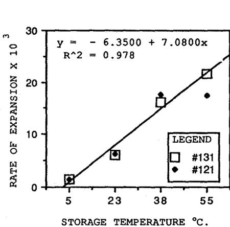
Figure 2. Effect of temperature on expansion of mortar bars made with two cements #131 and #121.
