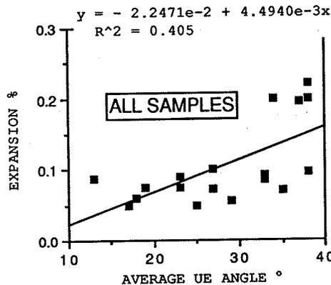
Figure 6b. Influence of UE angle in quartz grains in aggregates on the expansion of mortar bars. After Mullick [46]
