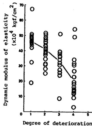
Fig. 4 Dynamic modulus of elasticity
