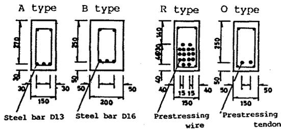
Fig.1 Outlines of the beam specimens
