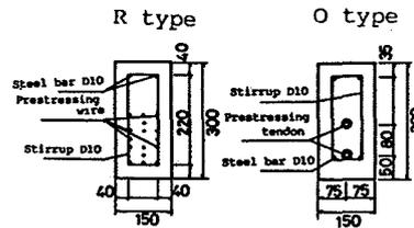
Fig.2 Outlines of the beam specimens
