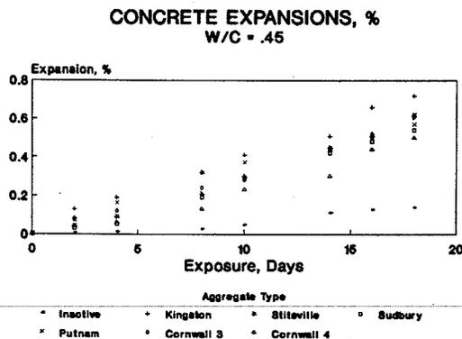
Fig. 2. AR Expansion of w/c 0.45 Concrete
