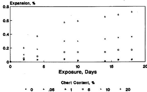
Fig. 5 AR expansion of mortar cores with different chert contents
