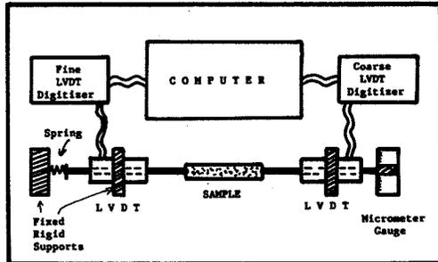
Fig. 1 Schematic Diagram of The Double LVDT Length Measuring Equipment
