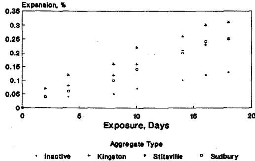
Fig. 3. AR Expansion of w/c 0.55 Concrete
