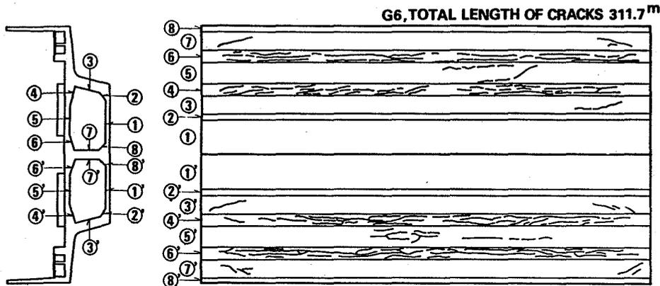
Fig-2 Crack illustration of the inner wall of the girder box
