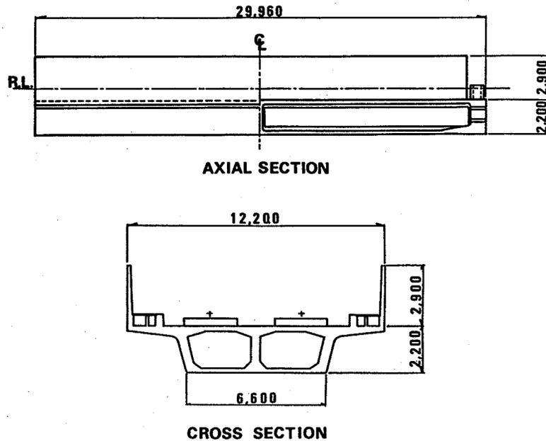
Fig-1 Dimensions of the girders
