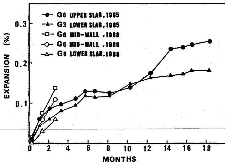
Fig-6 Expansion measurement
