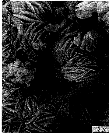
FIG. 3 ROSETTE-LIKE CRYSTALS IN THE WHITE INNER RIM DEPOSITS ON A REACTED SLATE AGGREGATE (B-90)
