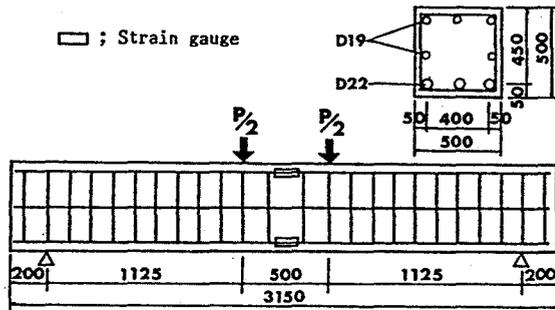
Figure 1 Cross-section of reinforced concrete beam
