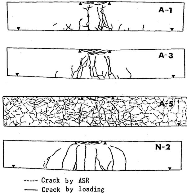
Figure 5 Failure mode
