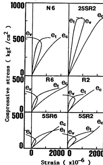
Fig.6 Relationship between compressive stress and strains
