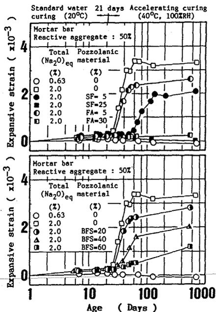
Fig.1 Expansive strains of mortar bars including pozzolanic materials
