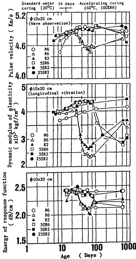
Fig.4 Results of non-destructive tests of silica fume concrete specimens
