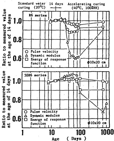
Fig.5 Correlation between results of non-destructive tests of concrete specimens and age
