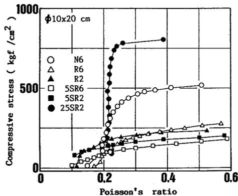
Fig.7 Relationship between compressive stress and Poisson's ratio
