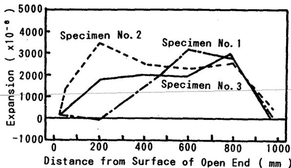
Figure-3-2 Distribution of Expansion with Axial Direction Gages
