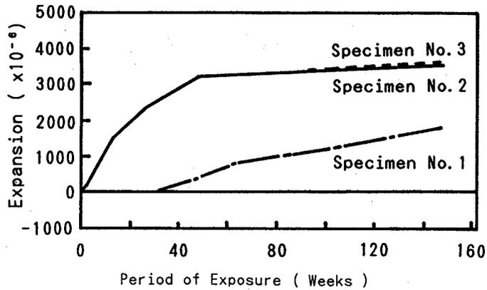
Figure-2-2 Expansion of Interior ( Average of 600mm and 800mm Depth )
