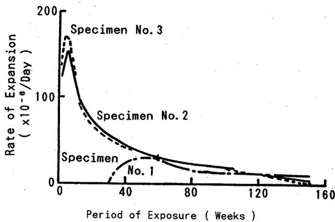
Figure-2-3 Rate of Expansion of Inside Concrete Dependent on Period of Exposure
