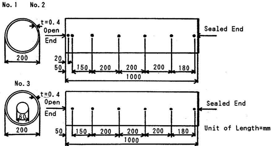
Figure-1 Detail of Model Specimens
