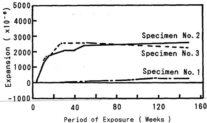
Figure-2-1 Expansion at 50mm Depth from Surface of Open End
