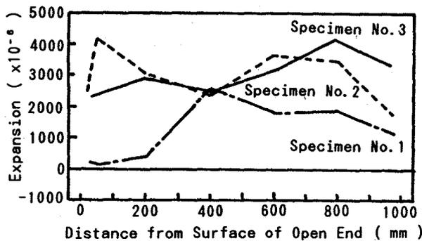
Figure-3-1 Distribution of Expansion with Radial Direction Gages
