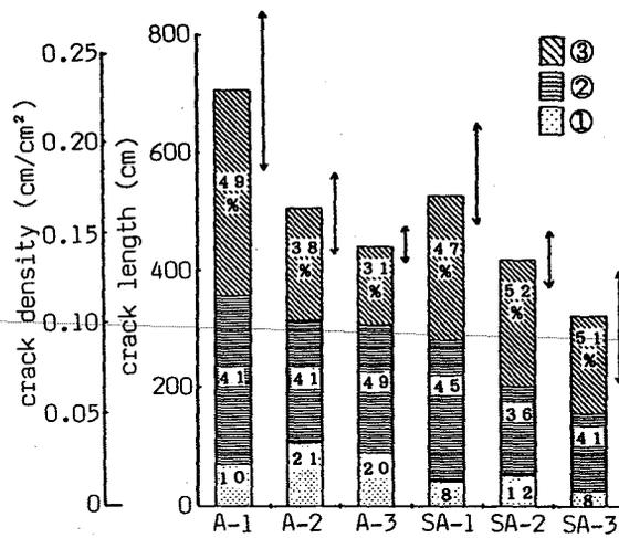
Fig. 5 Crack length and crack density (RC)
