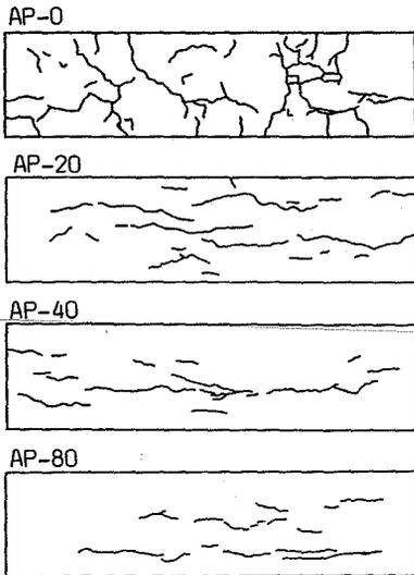
Fig. 4 Crack maps of PC specimens
