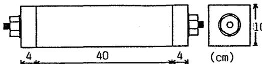
Fig. 2 Shape of PC specimen
