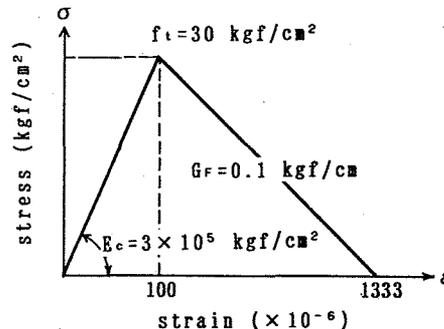
Fig. 11 Tensile stress strain curve
