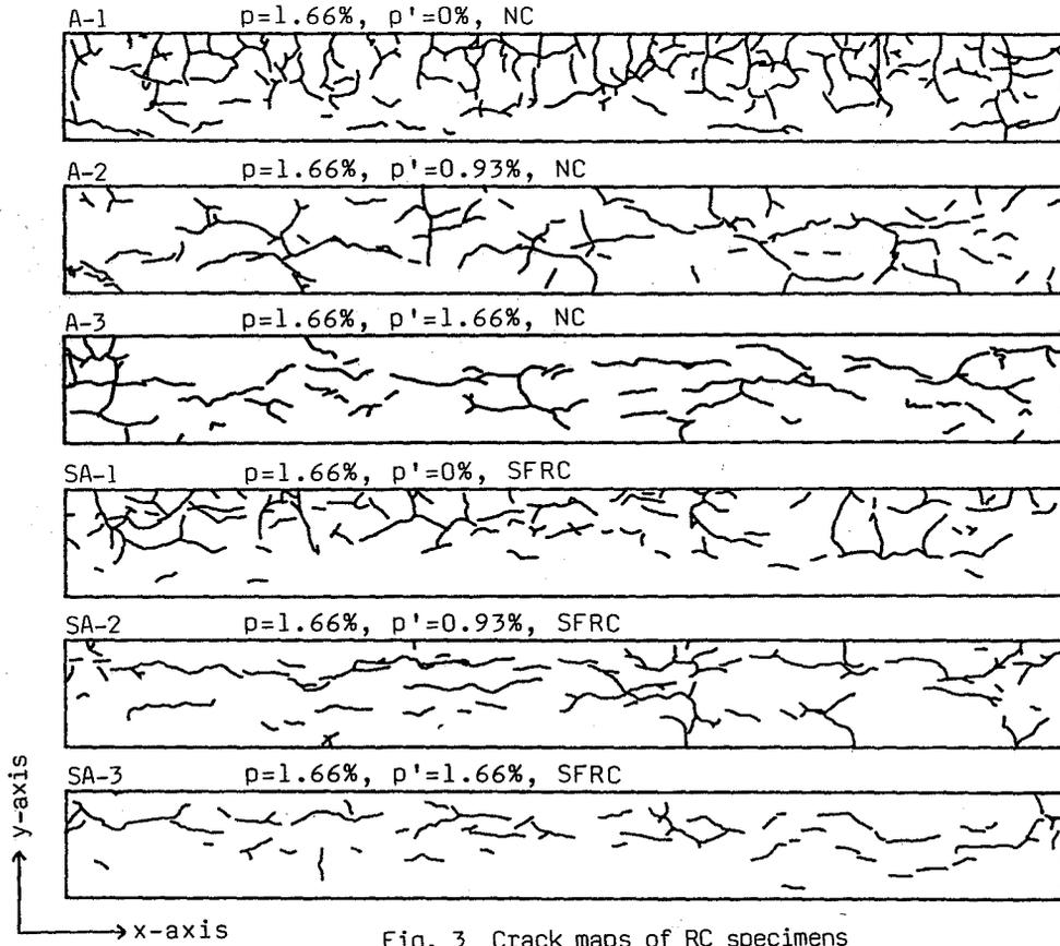
Fig. 3 Crack maps of RC specimens
