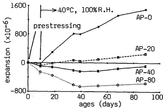
Fig. 9 Expansion of PC specimen
