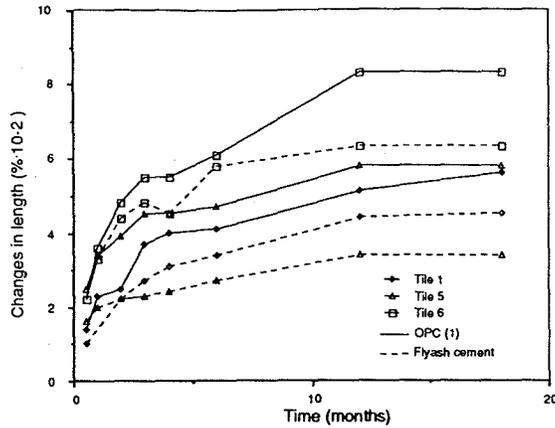
Fig 1 Changes in length of mortar prisms containing ceramic tiles as aggregate (ASTM C 227-81)
