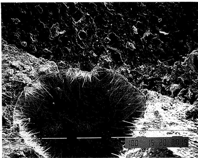
Fig 3 Crystal growth in mortar prisms
