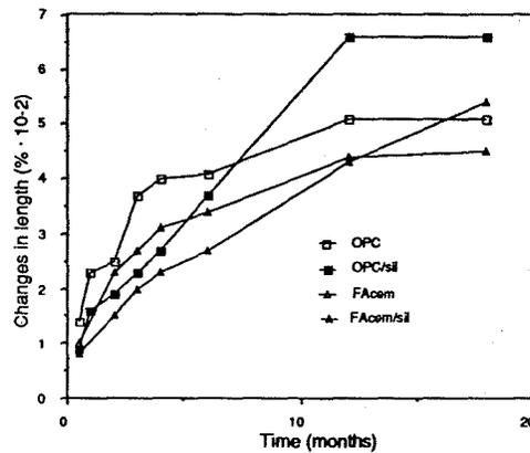
Fig 2 Changes in length of mortar prisms. Different types of cement with tile 1 as aggregate. (ASTM C 227-81)
