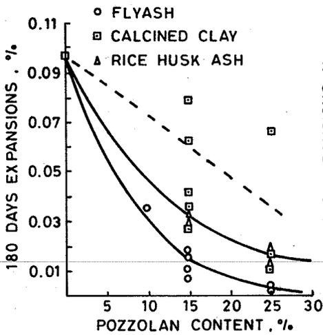
Fig. 5. Influence of pozzolan content - Natural aggregates (Series II)
