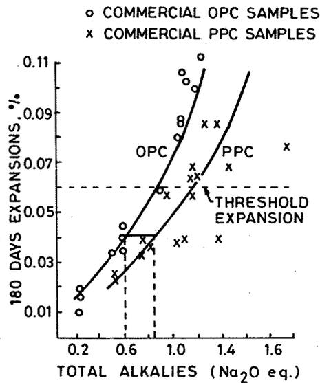
Fig. 4. Influence of alkali content in OPC or PPC samples. (Series I)
