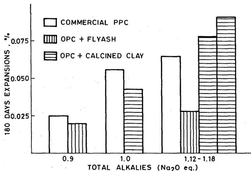
Fig. 7. Comparative performance of interground and blended pozzolans.
