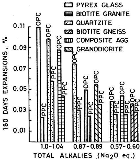
Fig. 3. Comparative performance of OPC and PPC samples. (Series I)
