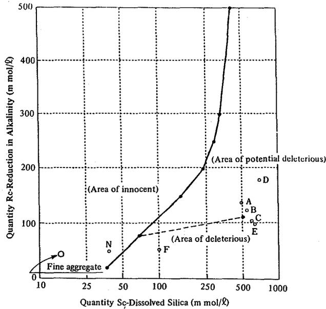
Fig. 1 Result of evaluation in accordance with ASTM evaluation method
