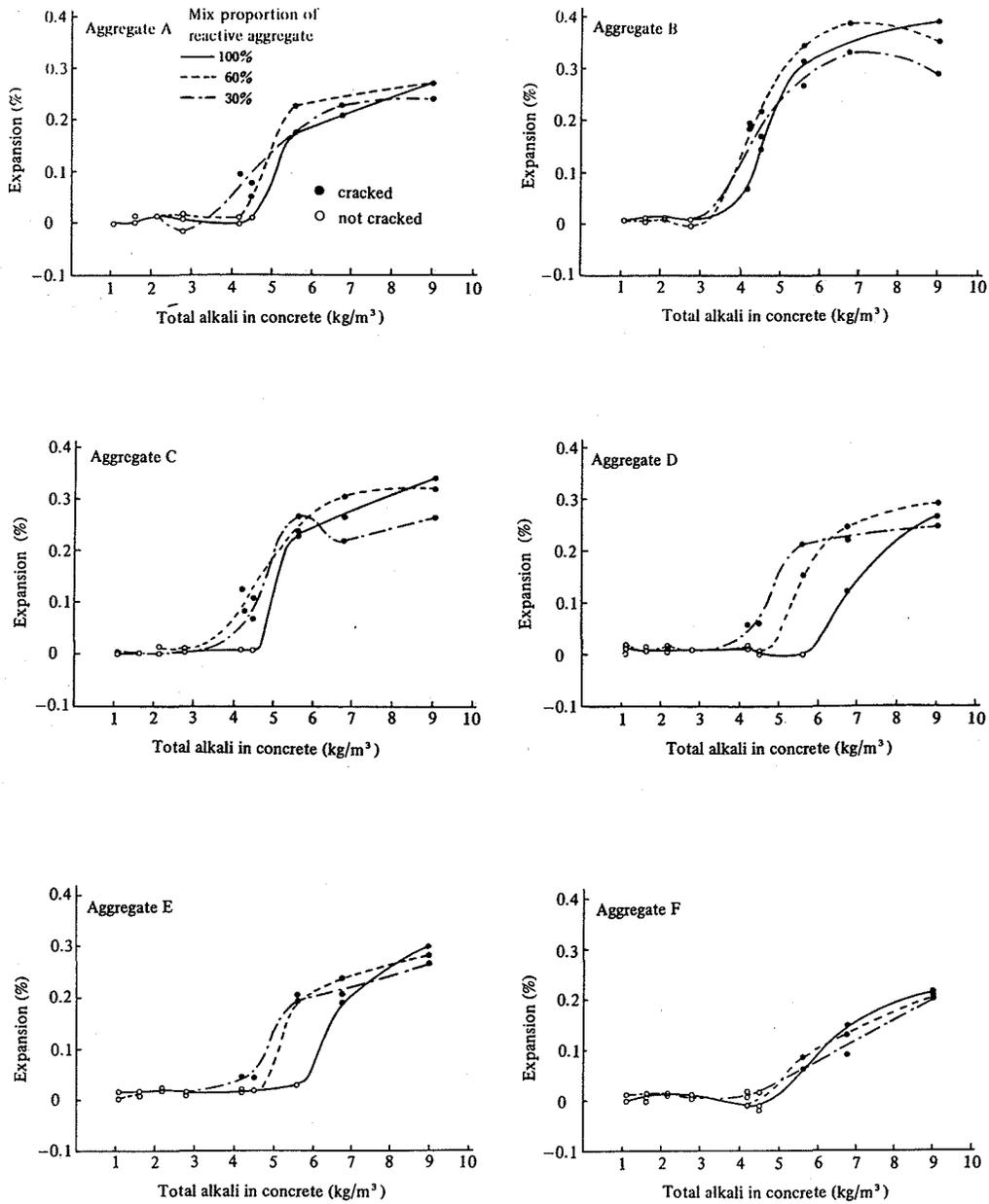
Fig. 2 Relation between total alkali in concrete and expansion
