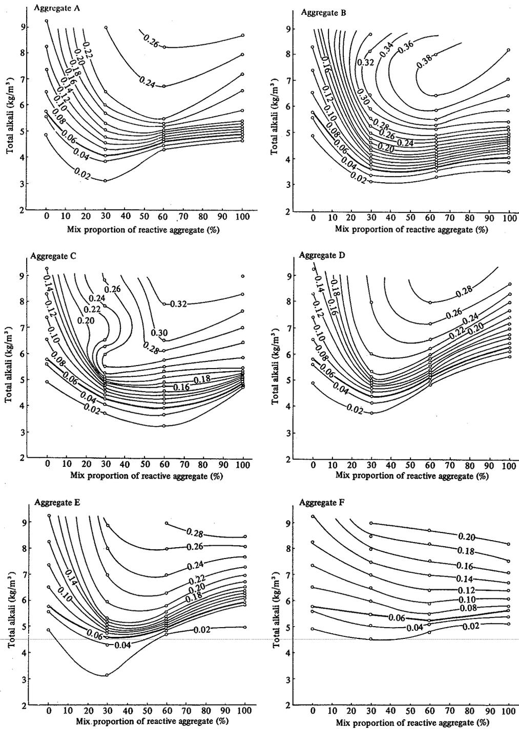
Fig. 3 Expansion contour line for reactive aggregate
