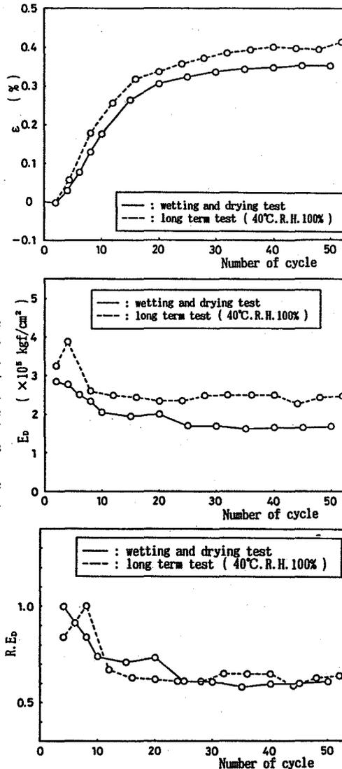
Fig.10 Relation between results of long-term test and wetting and drying test
