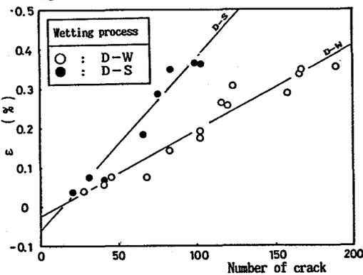
Fig. 6 Influence of immersed water (number of cracks)
