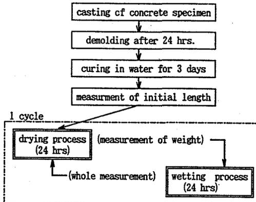
Fig.1 Condition of wetting and drying test
