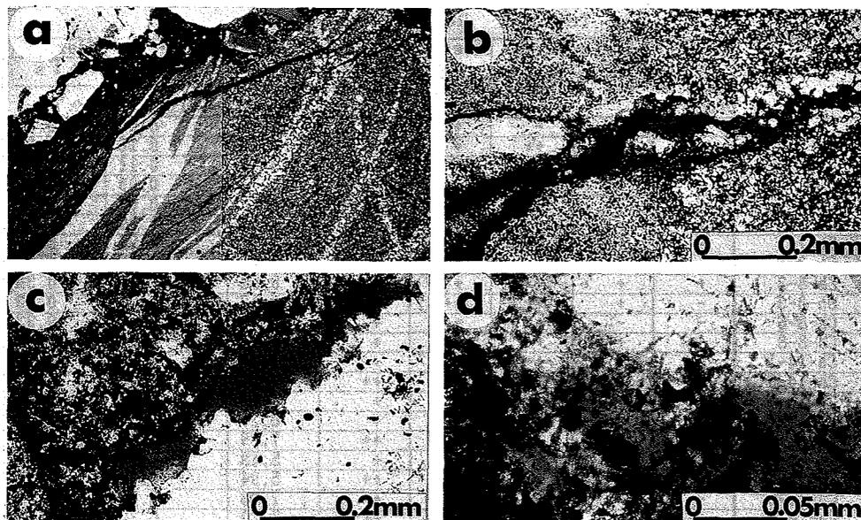
Photo 2 Products of the alkali-silica reaction on the boundaries between chert particle and cement paste and in the particle.
