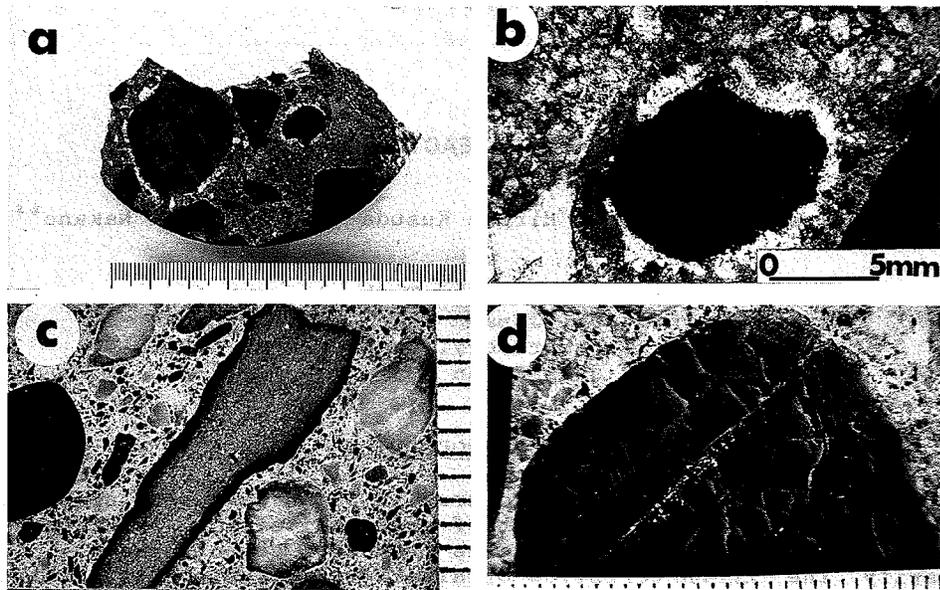
Photo 1. Products of the alkali-silica reaction in deteriorate concrete cores. a:A deteriorated concrete core(Sample Ch-16), b:Reaction products on the boundaries between chert particle and cement paste(Sample Ch-16-6), c:Dark rims in an alkali-reactive chert aggregate(Sample Ch-1-2), d:Reaction products in an alkali-reactive chert aggregate(Sample Ch-8-1).
