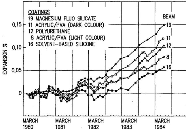
FIGURE 3: Dimensional change of large concrete beams made with alkali-reactive aggregate and high-alkali cement when exposed out of doors; different surface treatments had been applied about two months after casting
