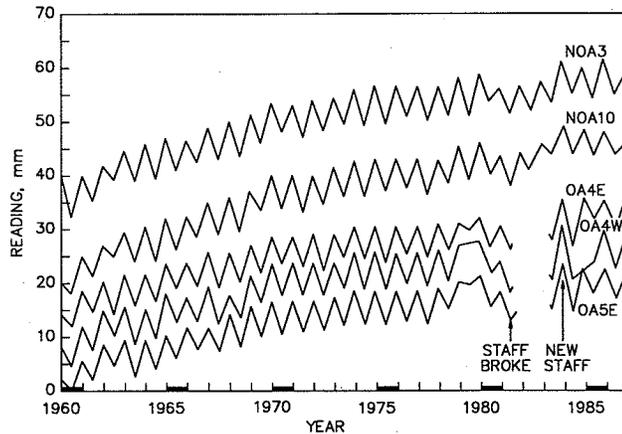
FIGURE 2: Some typical plots of long-term measurements taken on arches of the Churchill Dam
