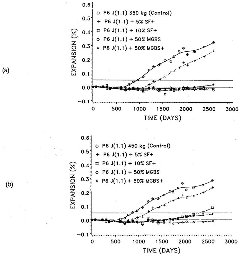
FIGURE 1: Graphs showing the effect of silica fume and milled granulated blast-furnace slag on the dimensional change of 300 mm concrete cubes made with alkali-reactive aggregate where the cement content was (a) 350 kg/m<sup>3</sup> and (b) 450 kg/m<sup>3</sup>
