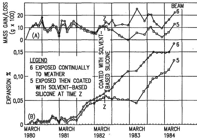
FIGURE 4: Effect of the application of a solvent-based silicone to a large concrete beam exposed outdoor and affected by asr with regard to (A) gain and loss of moisture, (B) dimensional change
