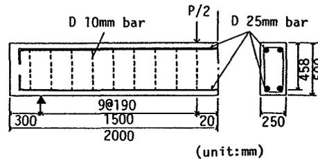
Figure 1. Beam specimen
