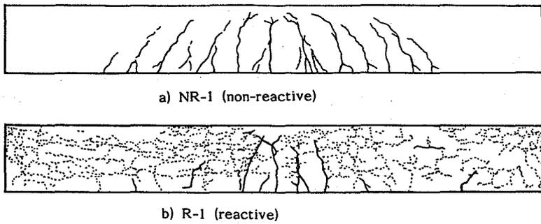
Figure 4. Crack pattern of the loaded beams
