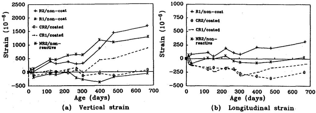
Figure 3. Concrete strain after coating
