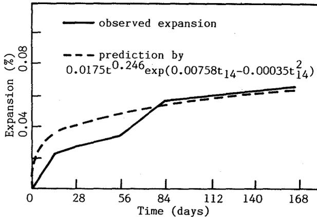
Fig. 5 Expansion of the reactive andesite and a predicted from the two-week measurement.
