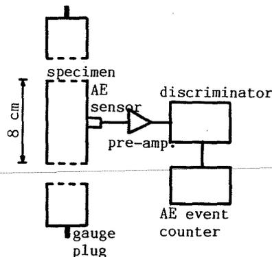
Fig. 3 Uniaxial compressive test of a mortar-bar specimen.
