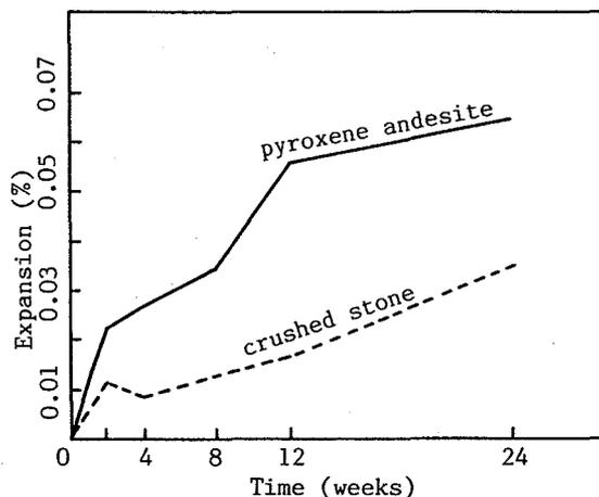
Fig. 1 Results of mortar bar tests for reactive and non-reactive aggregates.
