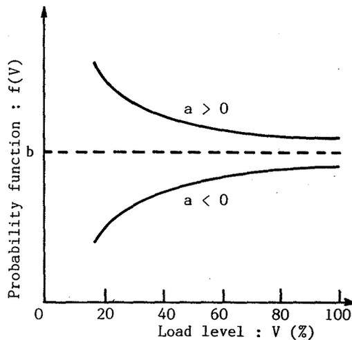
Fig. 2 Relations between probability function  $f(V)$  and load level  $V$  (%) in the rate process.
