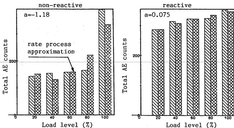
Fig. 4 AE activity in the uniaxial compressive tests of mortar-bar specimens.
