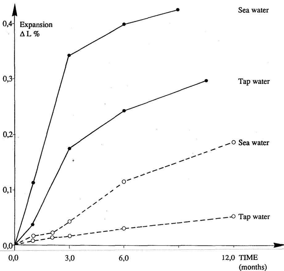
Fig. 2 The influence of sea water on mortar bar expansion due to alkali-silica reactions (Hvalfjord sand). [2]
