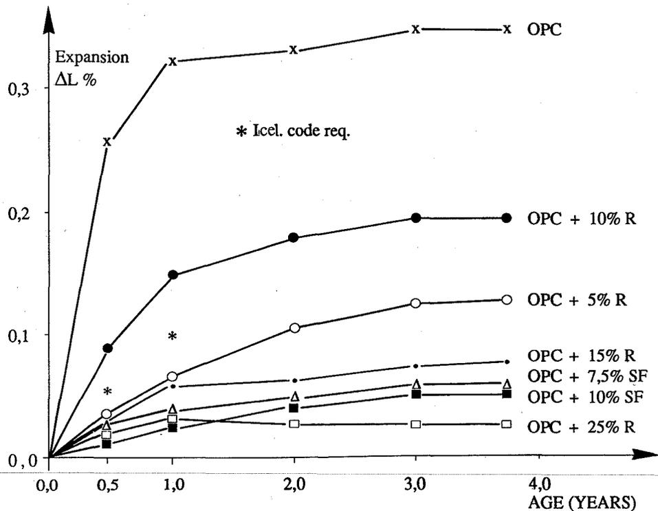
Fig. 1 Rhyolite (R) and silica fume (SF) vs. mortar bar expansion (Hvalfjord sand). [2]
