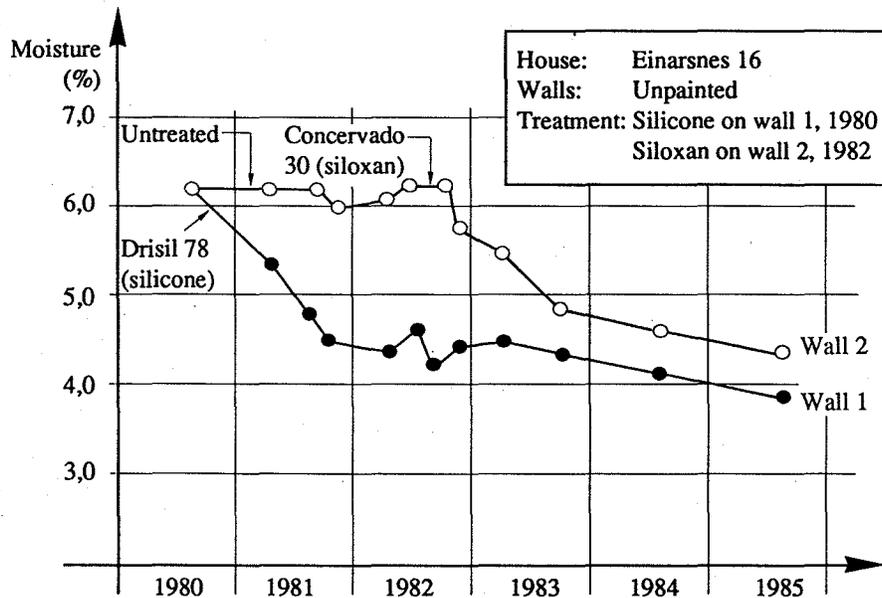
Fig. 3 Moisture development in concrete after impregnation with silicone (Disil 78 and siloxan (Conservado 30)). [14]
