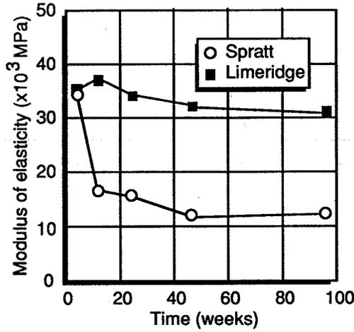
Figure 6 — Modulus of elasticity vs time for concretes stored in air at 38°C.
