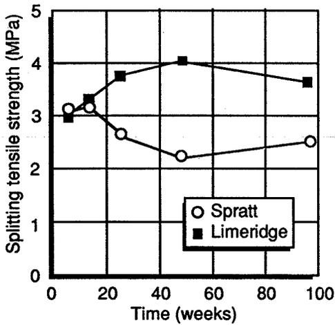
Figure 5 — Tensile strength vs time for concretes stored in air at 38°C.
