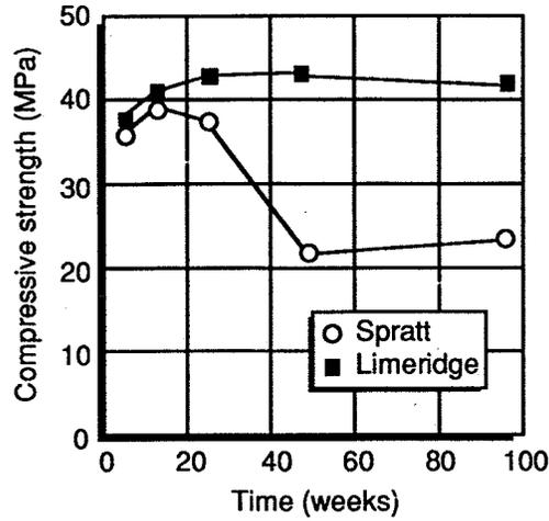
Figure 4 — Compressive strength vs time for concretes stored in air at 38°C.
