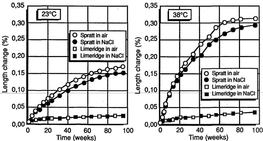
Figure 1 — Length changes (longitudinal expansions) of concrete specimens vs time.
