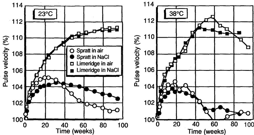
Figure 2 — Ultrasonic pulse velocity (PUNDIT) in concrete prisms (% of initial value) vs time.
