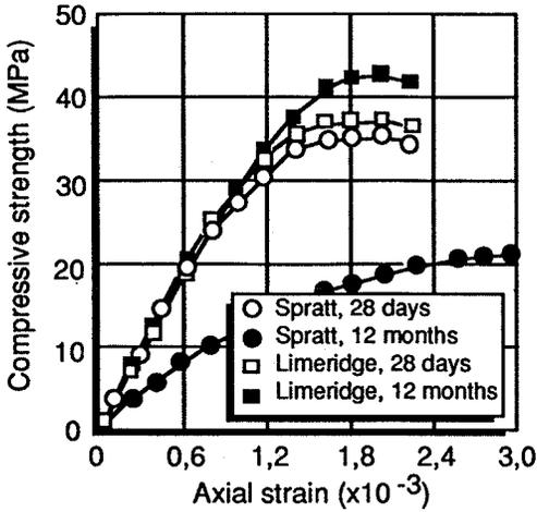
Figure 3 — Typical stress-strain curves for concretes stored in air at 38°C.
