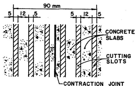
Fig. 6 - Joint Cutting with 6 Steel Wires
