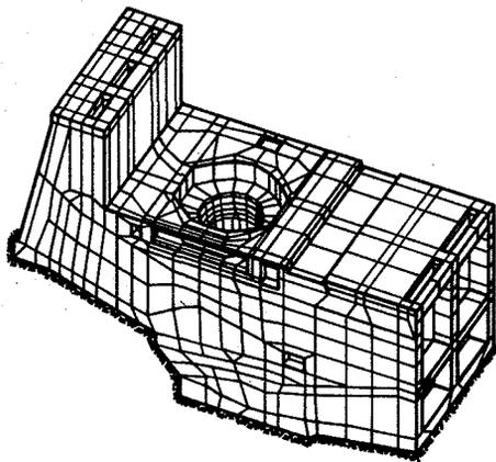
Fig. 2 - Finite Element Model
