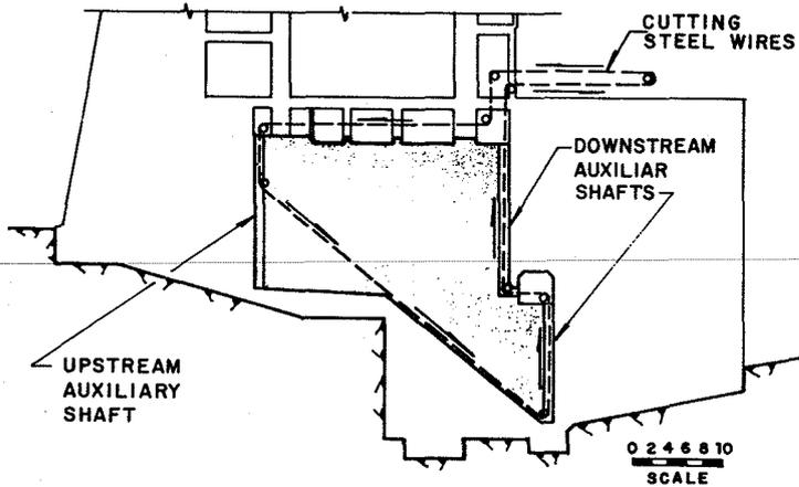
Fig. 5 - Cutting Area in a Contraction Joint
