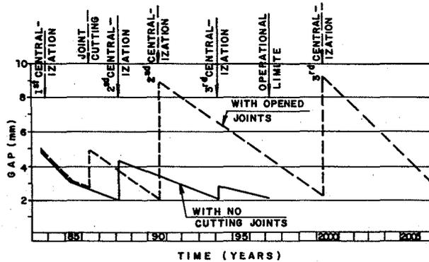
Fig. 4 - Gap Evolution in Friction Area of Unit 3
