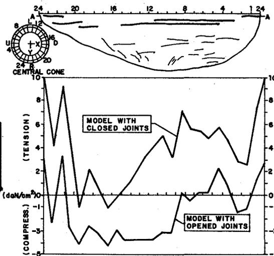
Fig. 3 - Cracks and Stresses at the Stay Vanes
