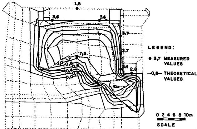
Fig. 7 - Joint Displacements After Cutting
