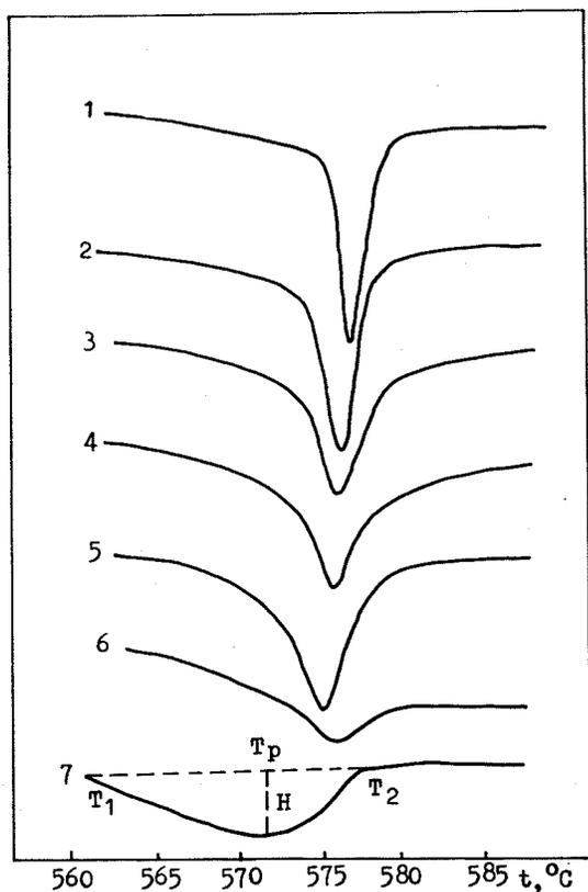
Fig.2 DSC, 1. quartz, 2. quartz, 3. microcrystalline quartz, 4. microcrystalline quartz and chalcedony, 5. chalcedony and microcrystalline quartz, 6. chalcedony, 7. chalcedony and microcrystalline quartz.
