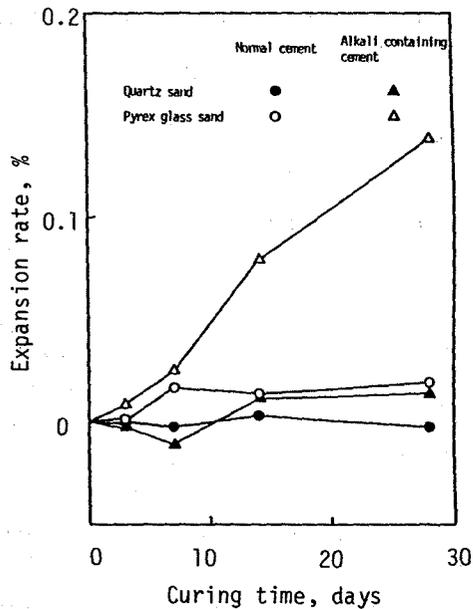
Fig. 2. Expansion characteristics of mortars.
