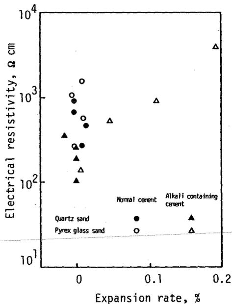
Fig. 4. Comparison of expansion and electrical resistivity of mortars.
