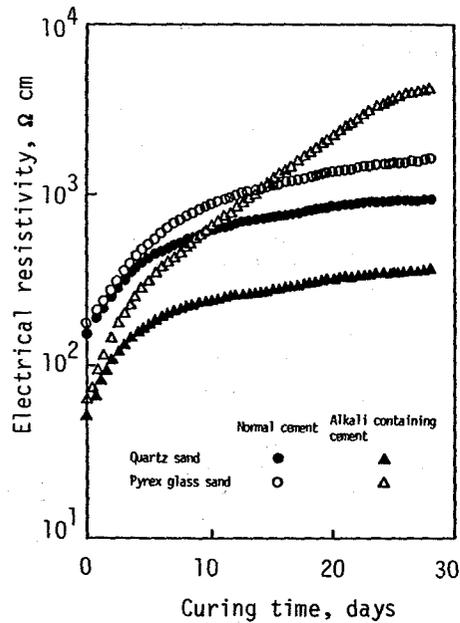
Fig. 3. Variation of electrical resistivity of mortars.
