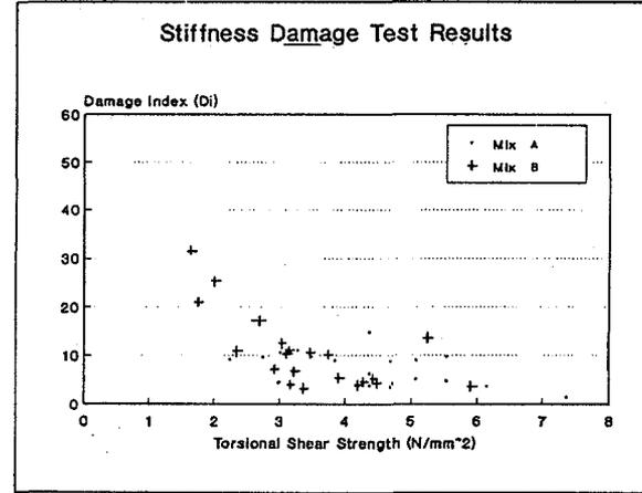
4. Comparison of Damage Index and Torsional Shear Strength
