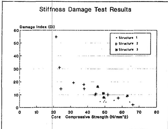
3. Comparison of Damage Index and Core Compression
