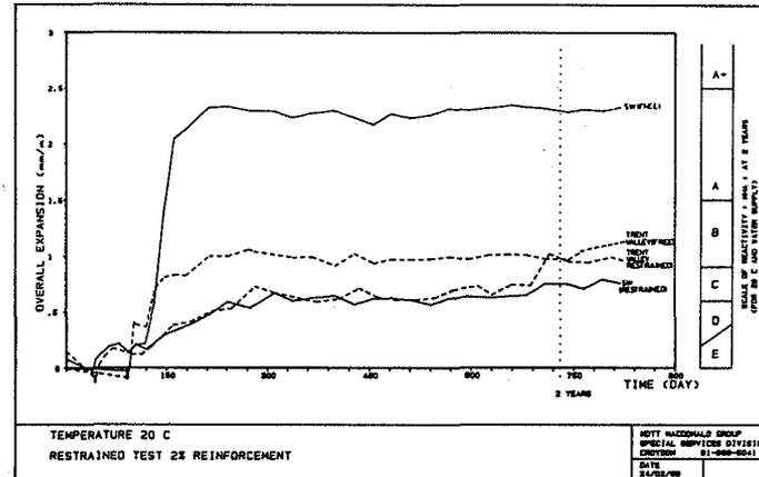
5. Comparison of Behaviour of different UK Aggregate Types
