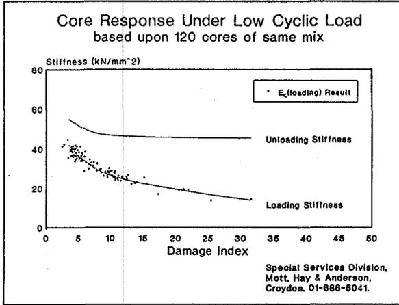
2. Comparison of  $E_c$  and Damage Index
