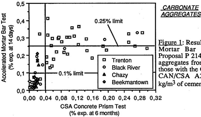
Figure 1: Results with the Accelerated Mortar Bar Method ASTM C-9 Proposal P 214 for quarried carbonate aggregates from Québec compared to those with the Concrete Prism Method CAN/CSA A23.2-14A (using 350 kg/m<sup>3</sup> of cement).
