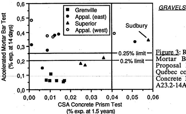
Figure 3: Results with the Accelerated Mortar Bar Method ASTM C-9 Proposal P 214 for gravels from Québec compared to those with the Concrete Prism Method CAN/CSA A23.2-14A.
