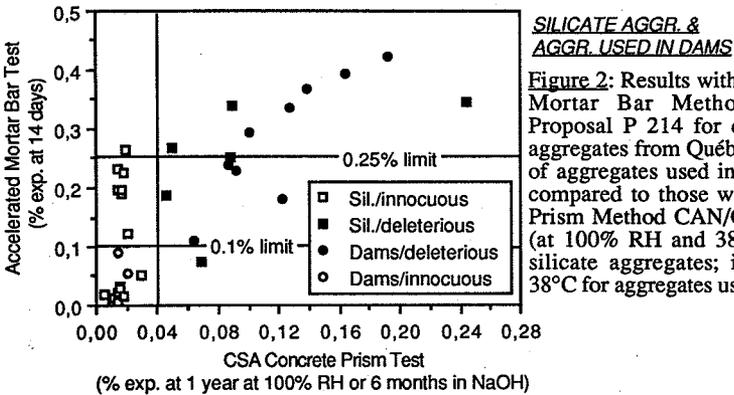
Figure 2: Results with the Accelerated Mortar Bar Method ASTM C-9 Proposal P 214 for quarried silicate aggregates from Québec and a number of aggregates used in Canadian dams compared to those with the Concrete Prism Method CAN/CSA A23.2-14A (at 100% RH and 38°C for quarried silicate aggregates; in NaOH 1N at 38°C for aggregates used in dams).
