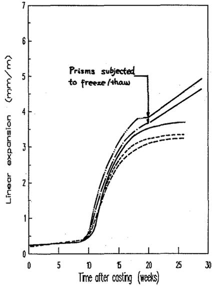
Figure 5 Expansion measurements of batch 1 concrete prisms
