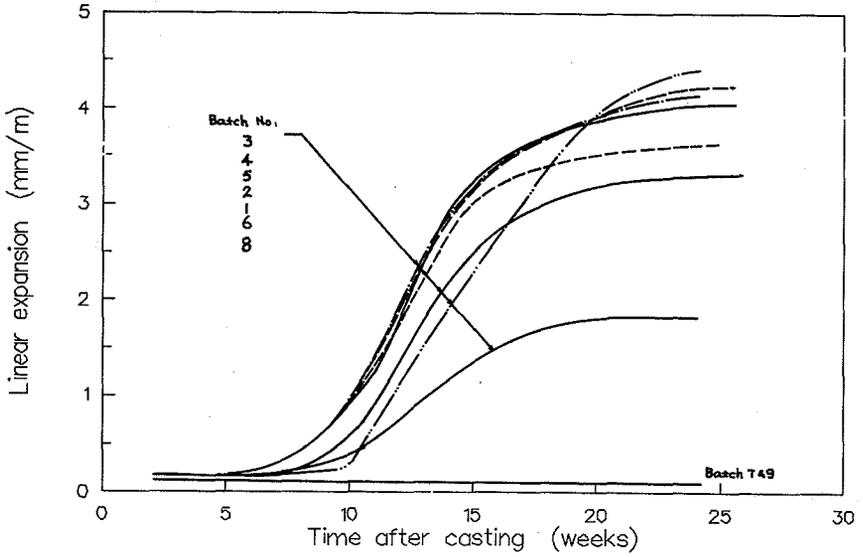
Figure 1 Batch average prism expansion measurements
