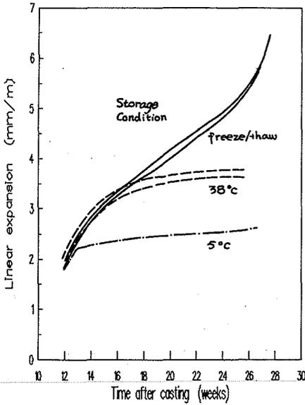
Figure 6 Expansion measurements of batch 2 concrete prisms
