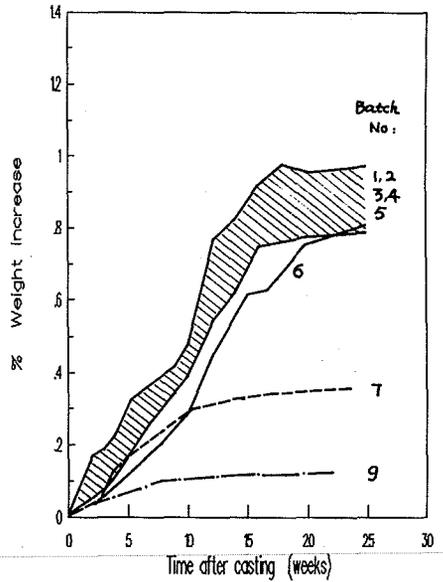
Figure 3 Batch average weight changes of concrete prisms
