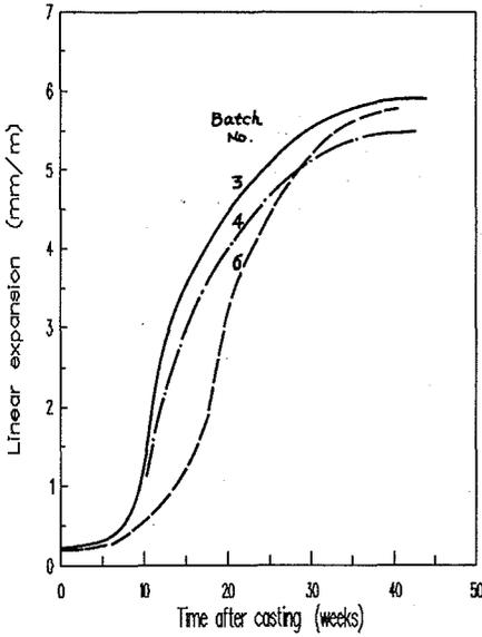
Figure 4 Batch average cylinder expansion measurements
