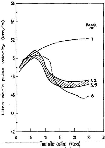
Figure 2 Batch average prism UPV measurements
