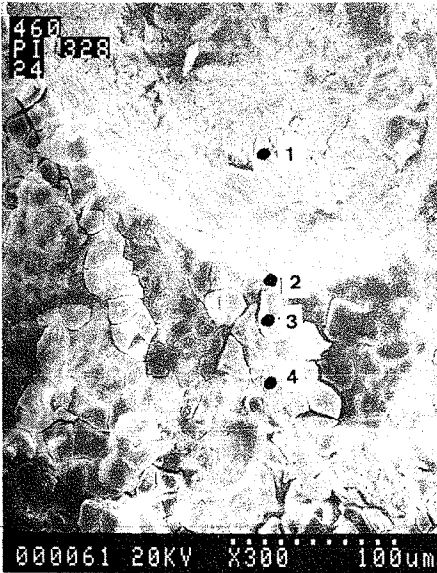
Figure 3 SEM micrograph of AAR gel associated with ettringite and thaumasite
