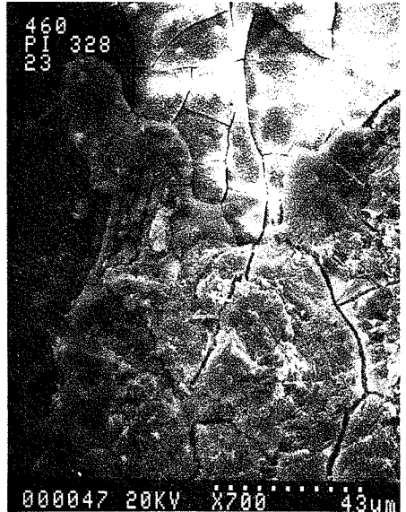
Figure 2 SEM micrograph of two separated gel layers
