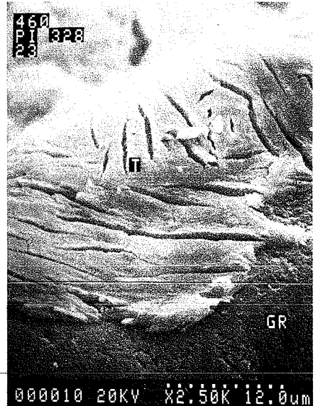
Figure 4 SEM micrograph of massive ettringite + thaumasite + calcite patch on a reactive aggregate
