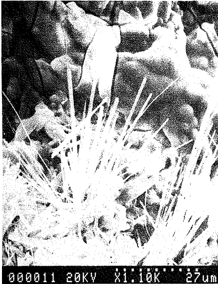
Figure 1 SEM micrograph of AAR gel associated with secondary ettringite
