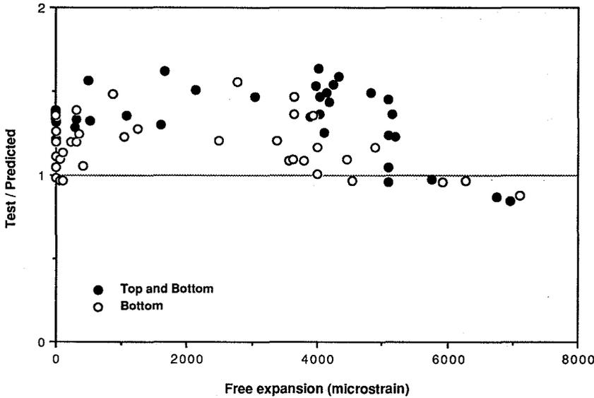
Figure 5. Punching strength ratio: two-phase theory.
