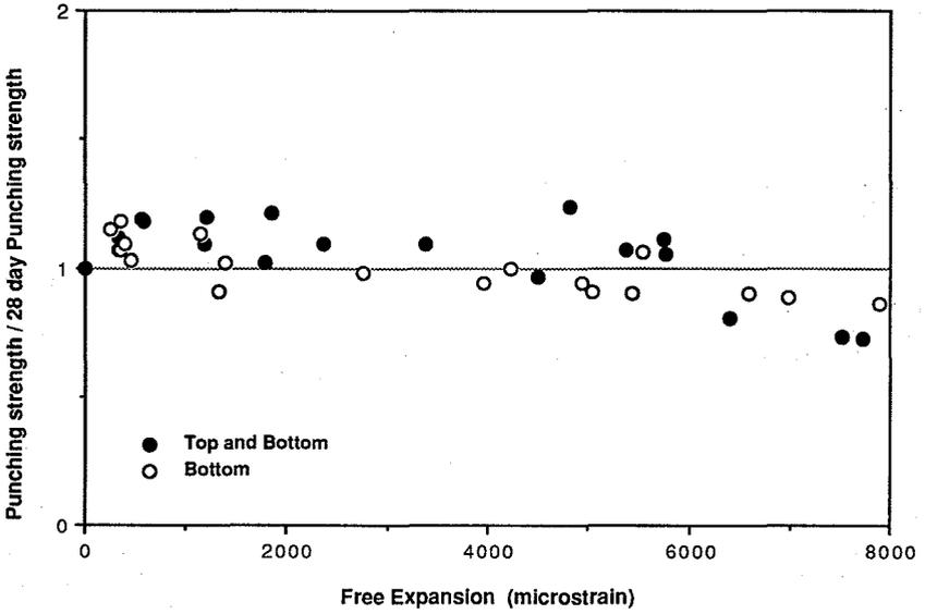
Figure 1. Effect of expansion on punching strength
