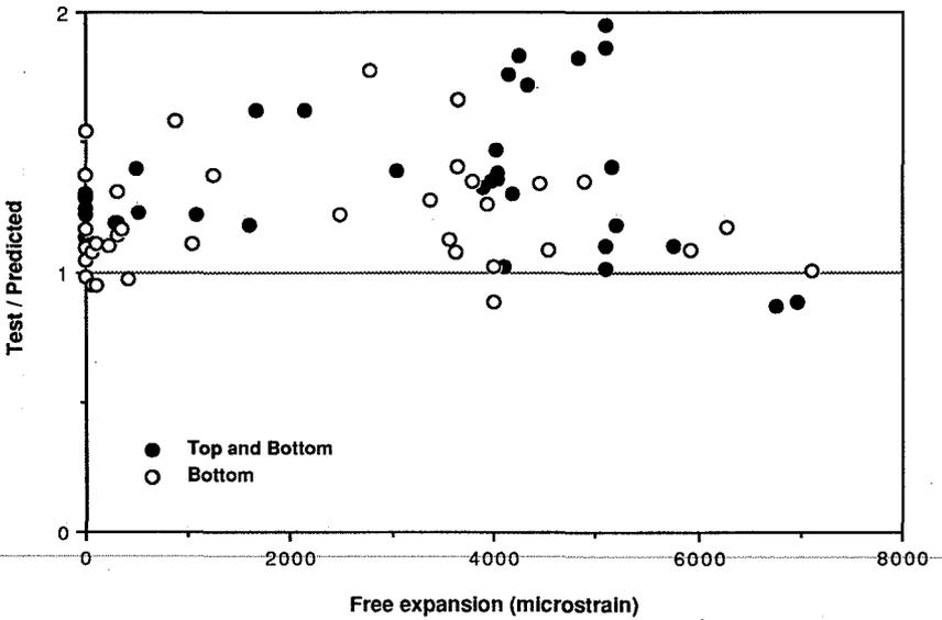
Figure 4. Punching strength ratio: decompression theory.
