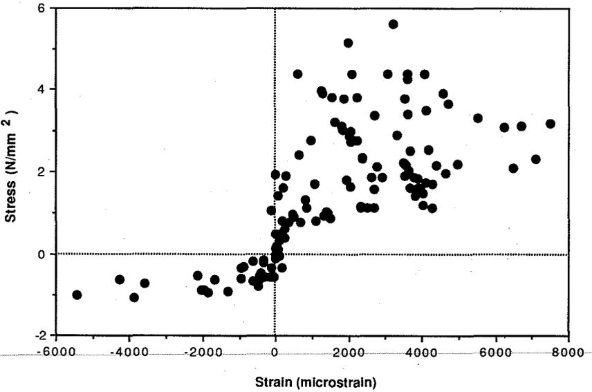
Figure 2. Slab surface concrete stresses and strains due to ASR
