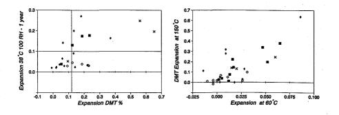
Figure 3. DMT expansions % versus mortar bar expansions % at 38°C
