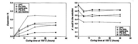
Figure 1. DMT expansion versus the duration of the cure (Spratt Agg.; b/a=2)
