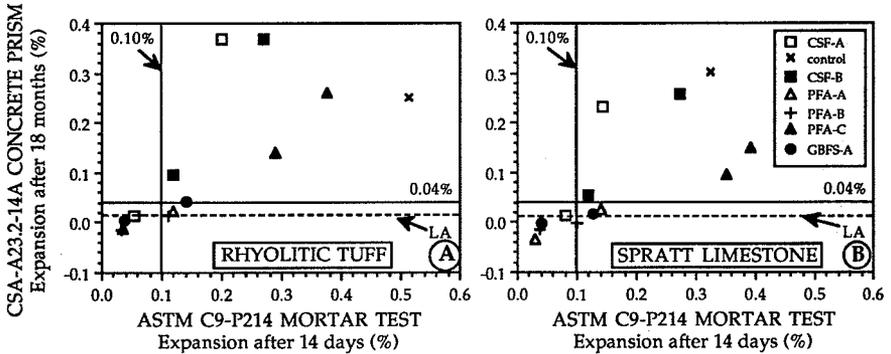
FIGURE 2 -- Relation between the expansion values at 18 months in the CSA concrete test and at 14 days in the ASTM test. A) Rhyolitic tuff B) Spratt limestone
