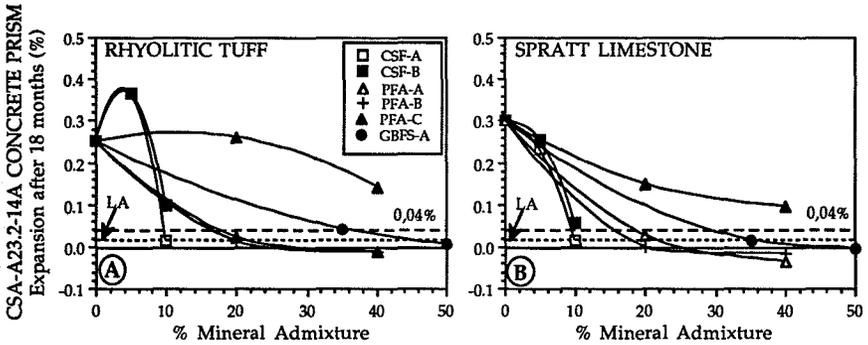
FIGURE 4 -- Expansion values measured at 18 months in the CSA-A23.2-14A concrete prism test as a function of the mineral admixture content. A) Rhyolitic tuff B) Spratt limestone
