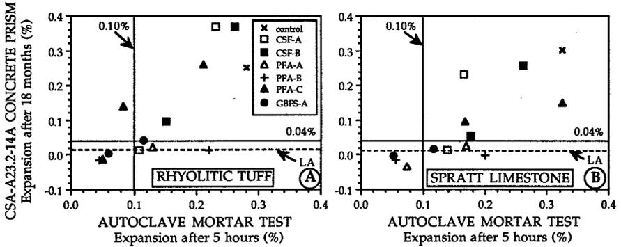
FIGURE 1 -- Relation between the expansion values at 18 months in the CSA concrete test and at 5 hours in the autoclave test. A) Rhyolitic tuff B) Spratt limestone
