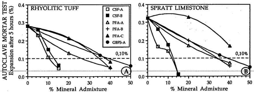
FIGURE 3 -- Expansion values measured at 5 hours in the autoclave mortar bar test as a function of the mineral admixture content. A) Rhyolitic tuff B) Spratt limestone
