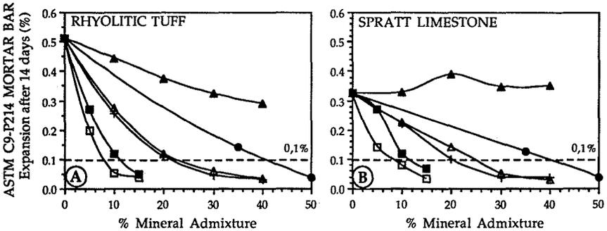
FIGURE 5 -- Expansion values measured at 14 days in the ASTM C9-P214 mortar bar test as a function of the mineral admixture content. A) Rhyolitic tuff B) Spratt limestone
