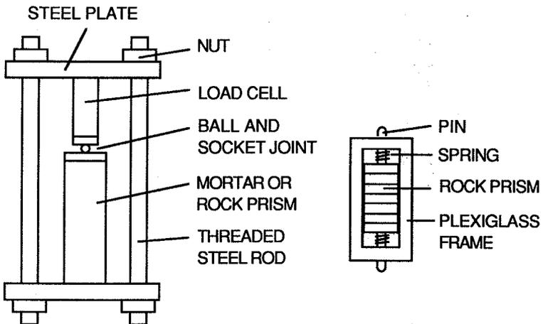
Fig. 2: Longitudinal confinement test assembly
