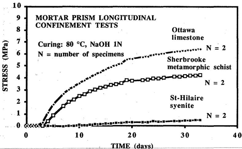
Fig. 9: Evolution of mortar prism longitudinal confinement stress
