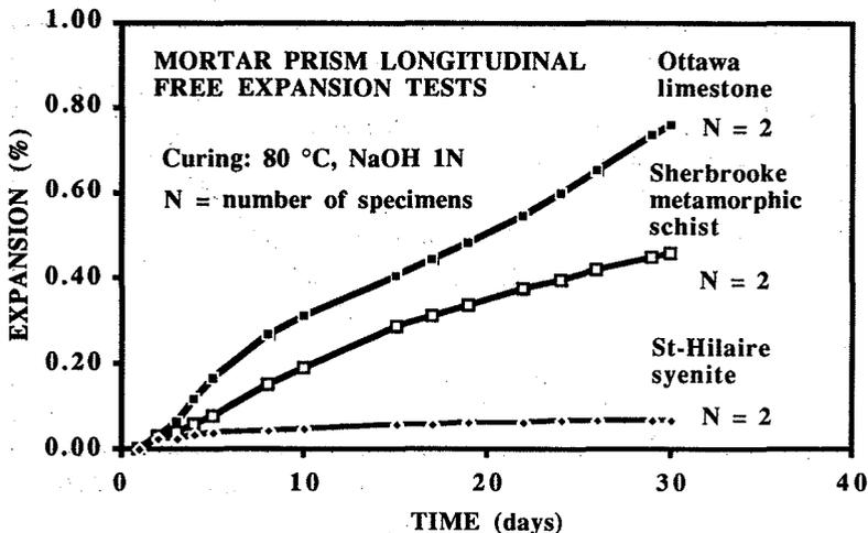
Fig. 8: Evolution of mortar prism free expansion
