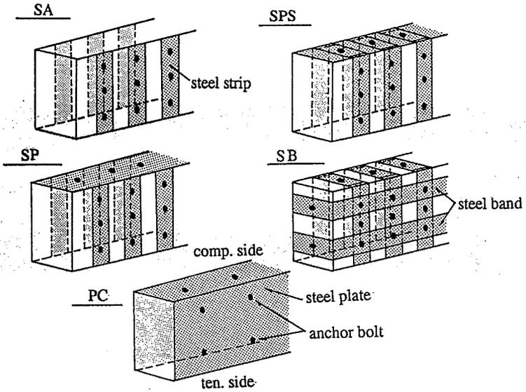
Figure 5 Reinforced specimens of Beam A
