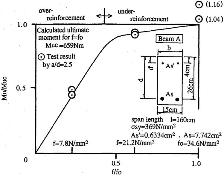
Figure 1  $M_u/M_{uc}$  vs  $f/f_o$  of Beam A ( $a/d=2.5$ )
