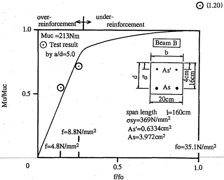
Figure 2  $M_u/M_{uc}$  vs  $f/f_o$  of Beam B ( $a/d=5.0$ )
